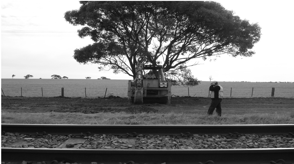
Figure 1. Photo during investigation of influence of a Black Box tree on rail track, Miram, Victoria, Australia
