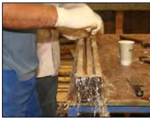
Figure 2: Fabrication process – layout on formwork
