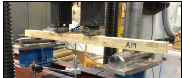
Figure 4: Four-point bending test setup
