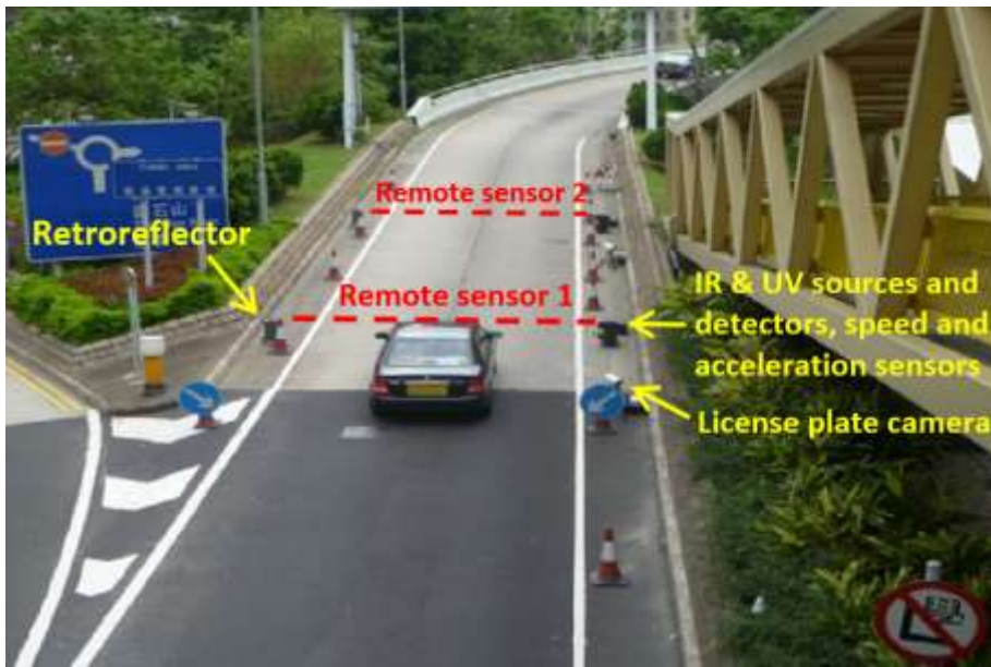
Fig. 1. Typical setup of on-road remote sensing measurement site.
