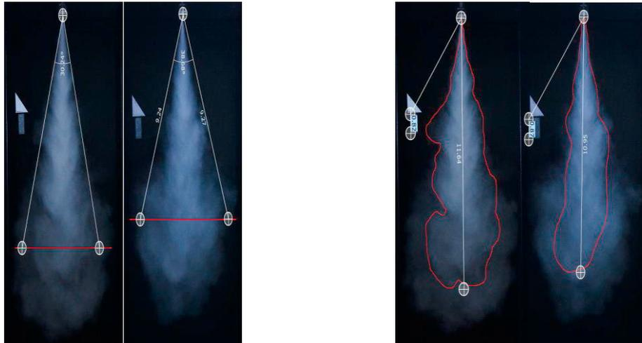
Fig. 2 (a) Spray angle of B100 (left) and distillate (right) at 0.4MPa. (b) Spray tip penetration of B100 (left) and distillate (right) at 0.4MPa.
