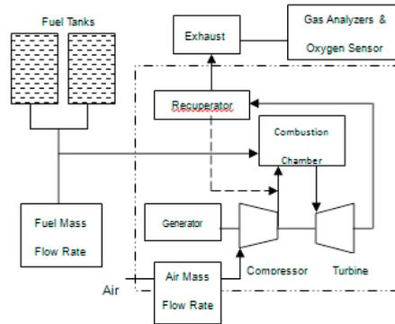
Fig. 1. Schematic diagram of the microturbine system.
