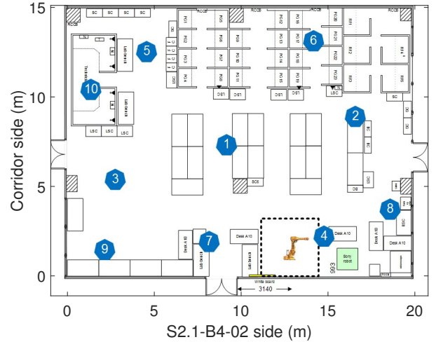
Fig. 2: 10 near-optimal sensor locations, ordered from most to least informative locations, in room S2.1-B4-01, Nanyang Technological University
