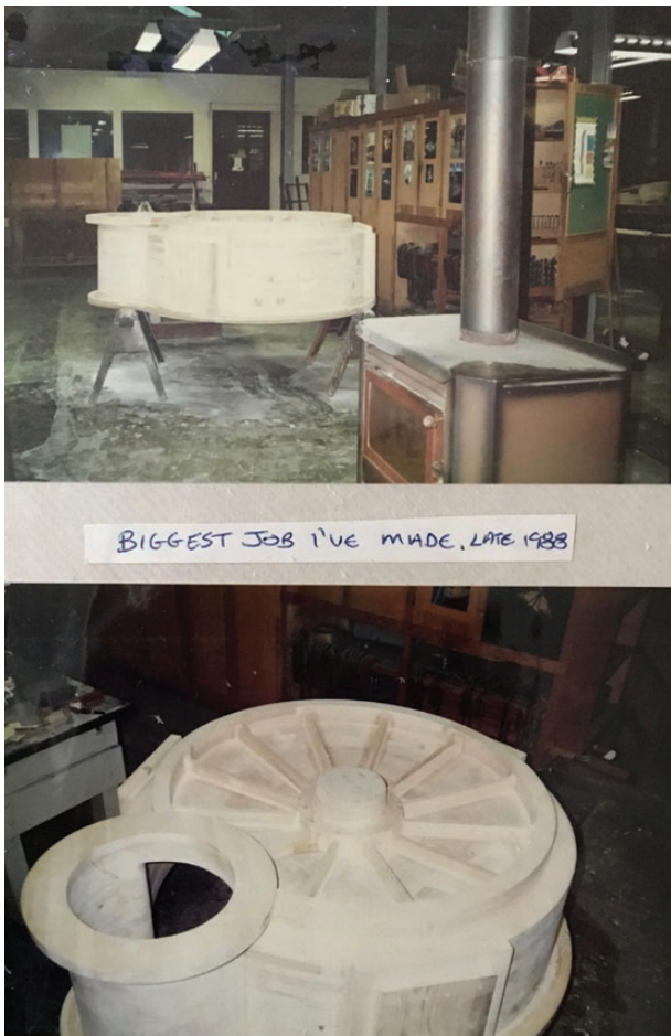
Fig 2. Large pattern for a casting by Debra Schuckar, State Electricity Commission Victoria, 1988, personal album, reproduced with permission.
