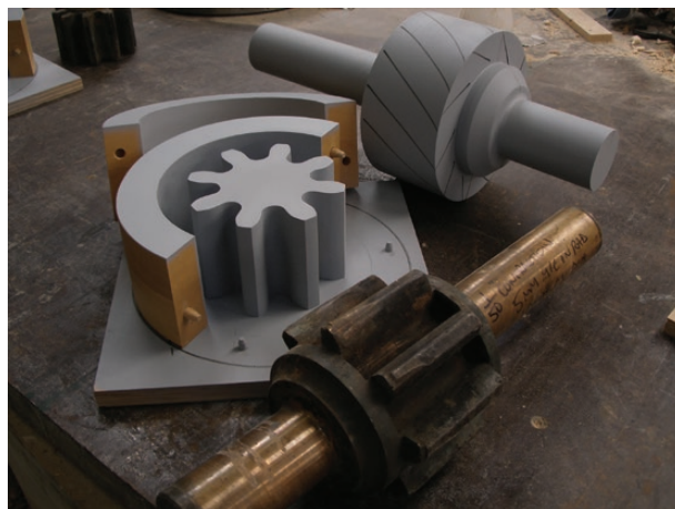
Fig 1. Gear pattern (with resultant casting) by Peter White, Dolman Pattern & Model Makers, n.d., reproduced with permission.
