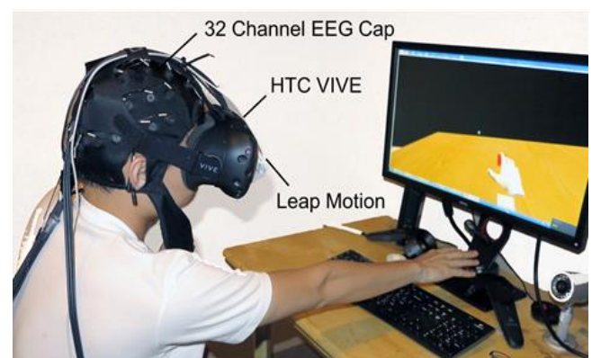
FIGURE 1. Our EEG-based experiment evaluated the interaction techniques in VR by measuring intentionally elicited cognitive conflict.
