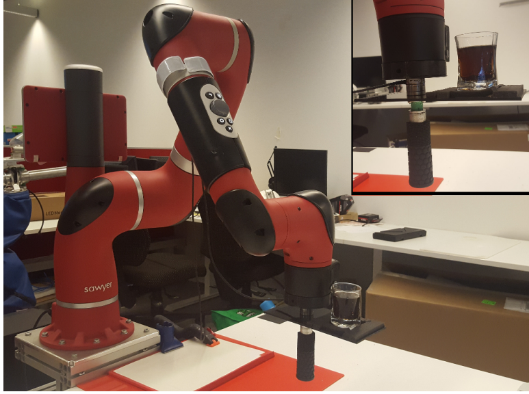
Fig. 3. Experimental setup: 7R serial manipulator with a force sensor rigidly attached to the robot end-effector, a tool that combines a joystick and a flat rectangular plastic tray of 190x95x3mm attached to the sensor and a shot glass with liquid.
