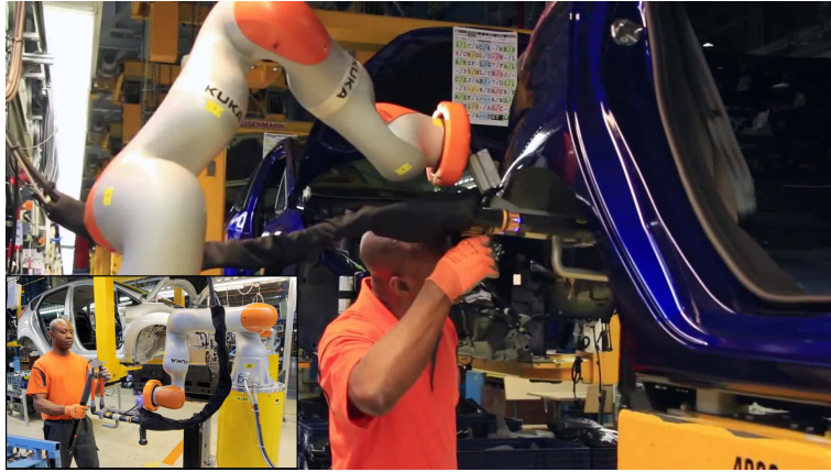
Fig. 1. Operator and robotic manipulator working side-by-side in Cologne (Germany) Ford’s factory (image courtesy of KUKA Robots Ibérica, S.A, Vilanova i la Geltrú, Spain).
