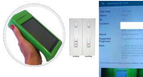
Figure 1. Example of an early custom prototype test strip analyser for malaria detection (Courtesy AusSI Systems).
