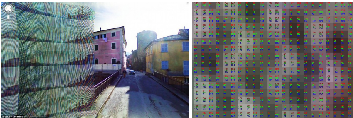
Fig. 1.6. Image of urban scene showing transmission or glitch error artefacts (left) and close-up of the artefact area in a PixelMath analysis showing numerical distribution of RGB pixel values (right). Left-hand image: Emilio Vavarelle. Google StreetView.
