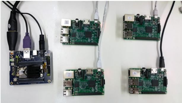
Fig. 8: Embedded IoT boards used for computer control.
