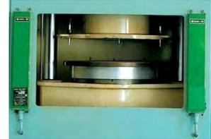
FIGURE 12. Testing machine of disc assembly.
