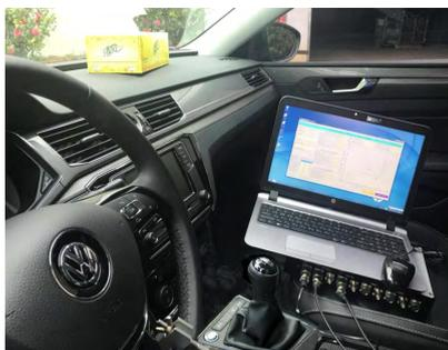
FIGURE 19. The testing bench of clutch pedal control.
