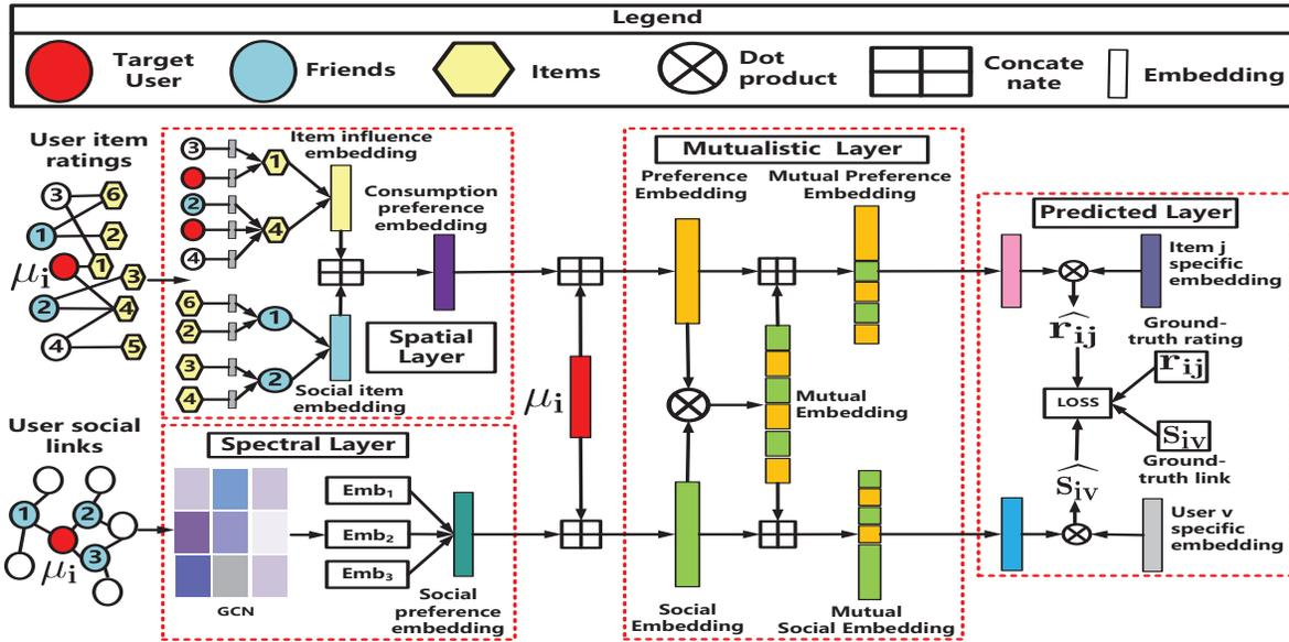
Fig. 2. The architecture of MGNN. It contains four components: spatial layer, spectral layer, mutualistic layer, and predicted layer.
