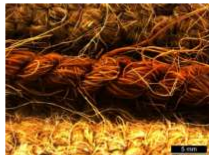
Figure 7 Internal observation under optical-microscope on jute filter and coconut cores indicates no soil clogging BPVDs
