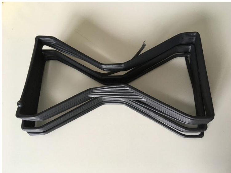
Figure 6. Shrinkage and bowing
