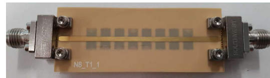
FIGURE 11. Fabricated filter with W_p = 6.5 mm, L_p = 3 mm, s = 1.25 mm, R_v = 0.125 mm and w = 1.5 mm.
