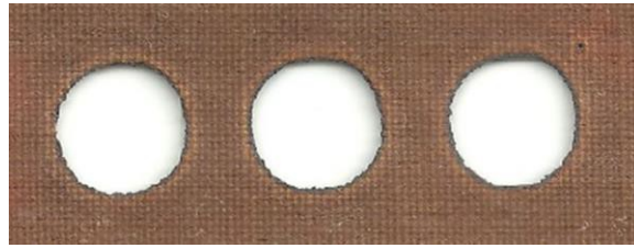
Fig. 9 - Sample holes drilled by diode laser
