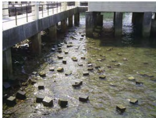
Figure 4: Concrete cubes exposed in the Gulf of Thailand [47]
