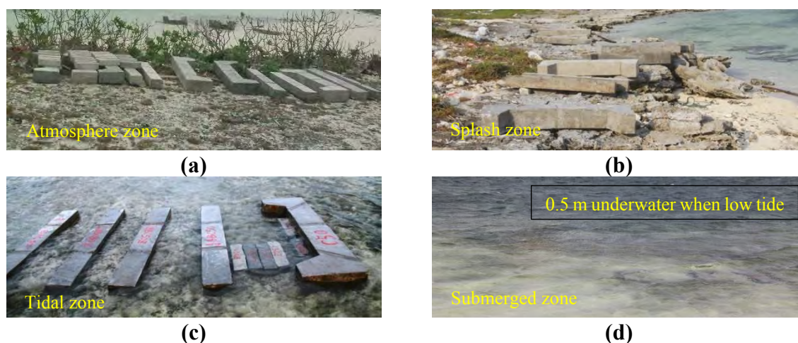
Figure 10: RC columns, RC beams and concrete prisms exposed on the island
