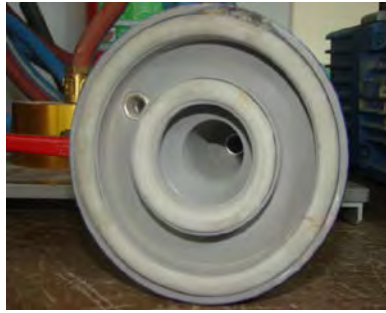
Figure1: Test chamber and external protection ring of the Torrent permeability tester.
