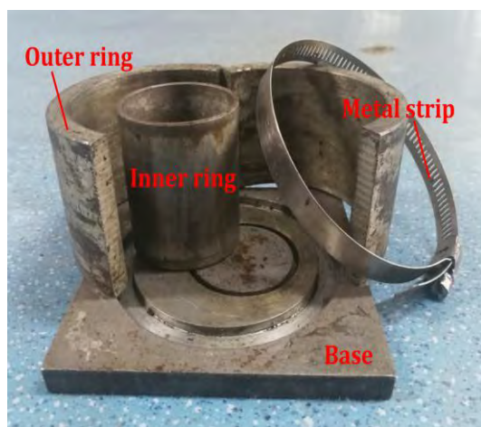
Figure 1: Actual mold of the eccentric ring test (left)
