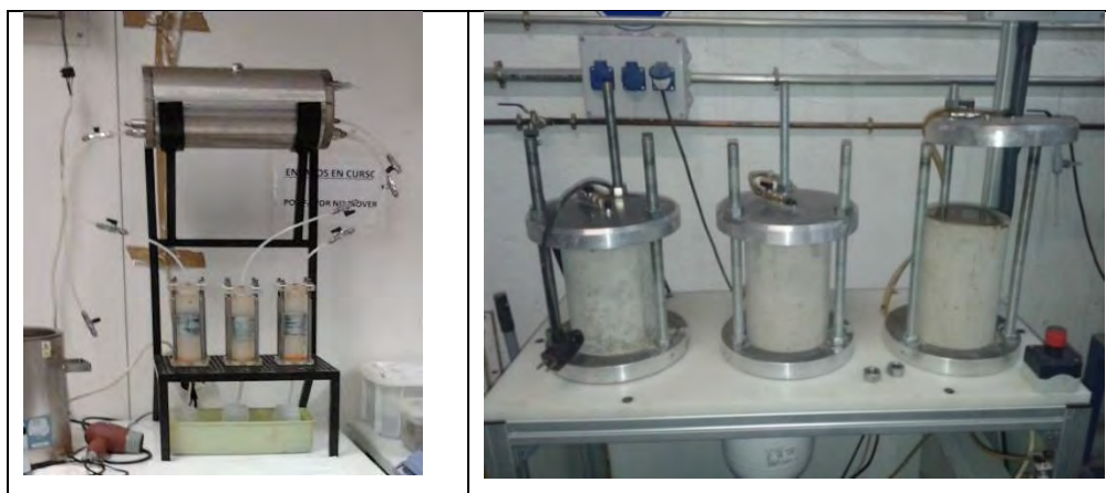
Figure 1: Left: Arrangement for percolation tests from the upper surface with pressures until 2,5bar. Machine for tests until 7 bars with water introduced by the lower face of the specimens
