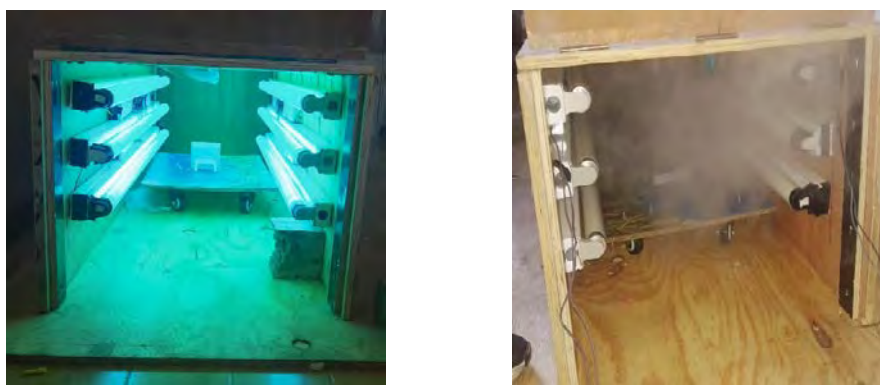
Figure 1: The home-made ageing box
