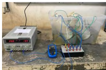
Figure 2: Chloride chloride migration test in progress
