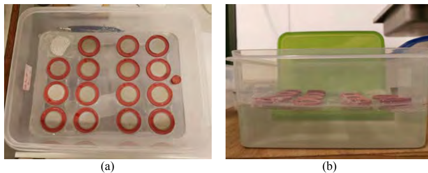
Figure 1: The setup for unidirectional sulfate penetration test
