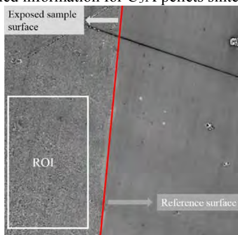
Figure 3: Morphology of partial polished C_3A pellet in phase image obtained by DHM. Reference surface is the surface covered by platinum player. The size of ROI (region of interest) is 220 pixel x 370 pixel, and the size of each pixel is 299 nm x 299 nm
