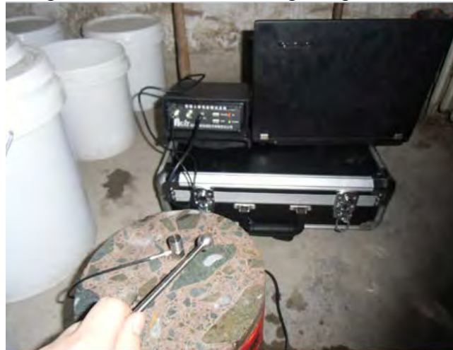
Figure 3: Elastic wave velocity testing device
