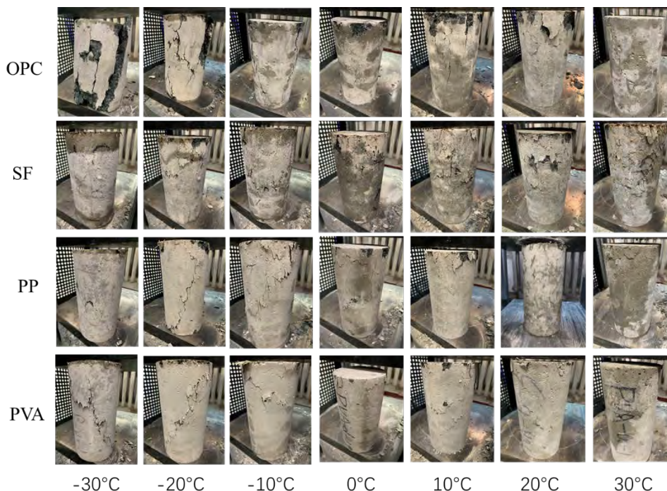
Figure 3: Failure mode of specimens
