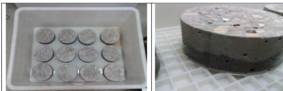
Figure 2: Left: samples submitted to water absorption. Right: detail of the rack and the level of the water
