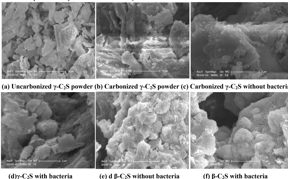
Figure 7: SEM micrographs of C 2 S with different carbonation conditions and magnification
