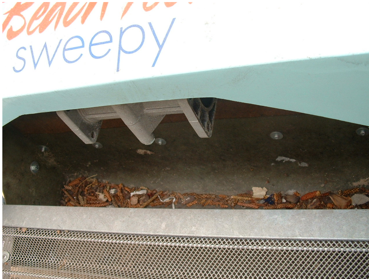
In-situ sieving using portable vibrating sieve
