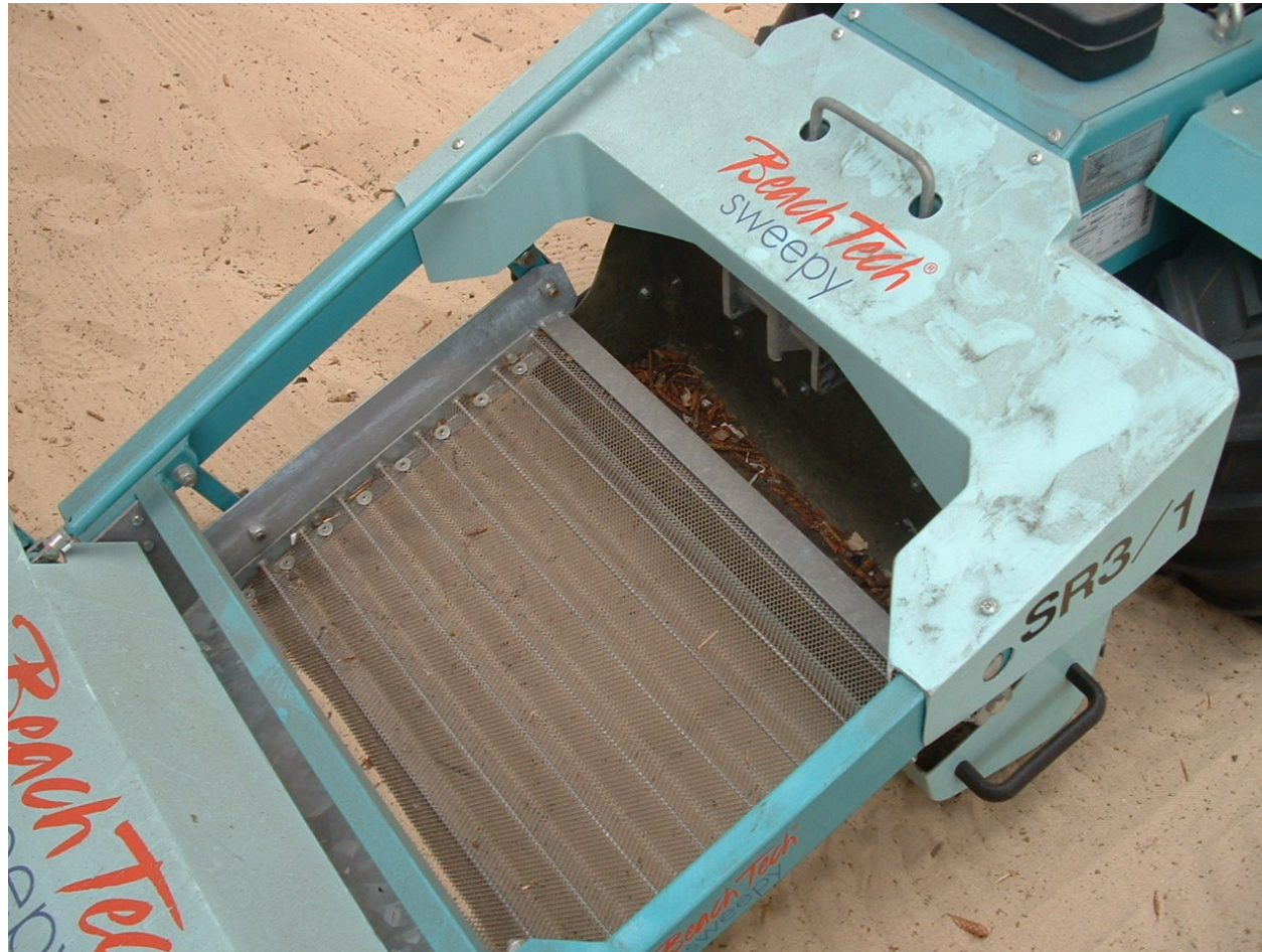
In-situ sieving using portable vibrating sieve
