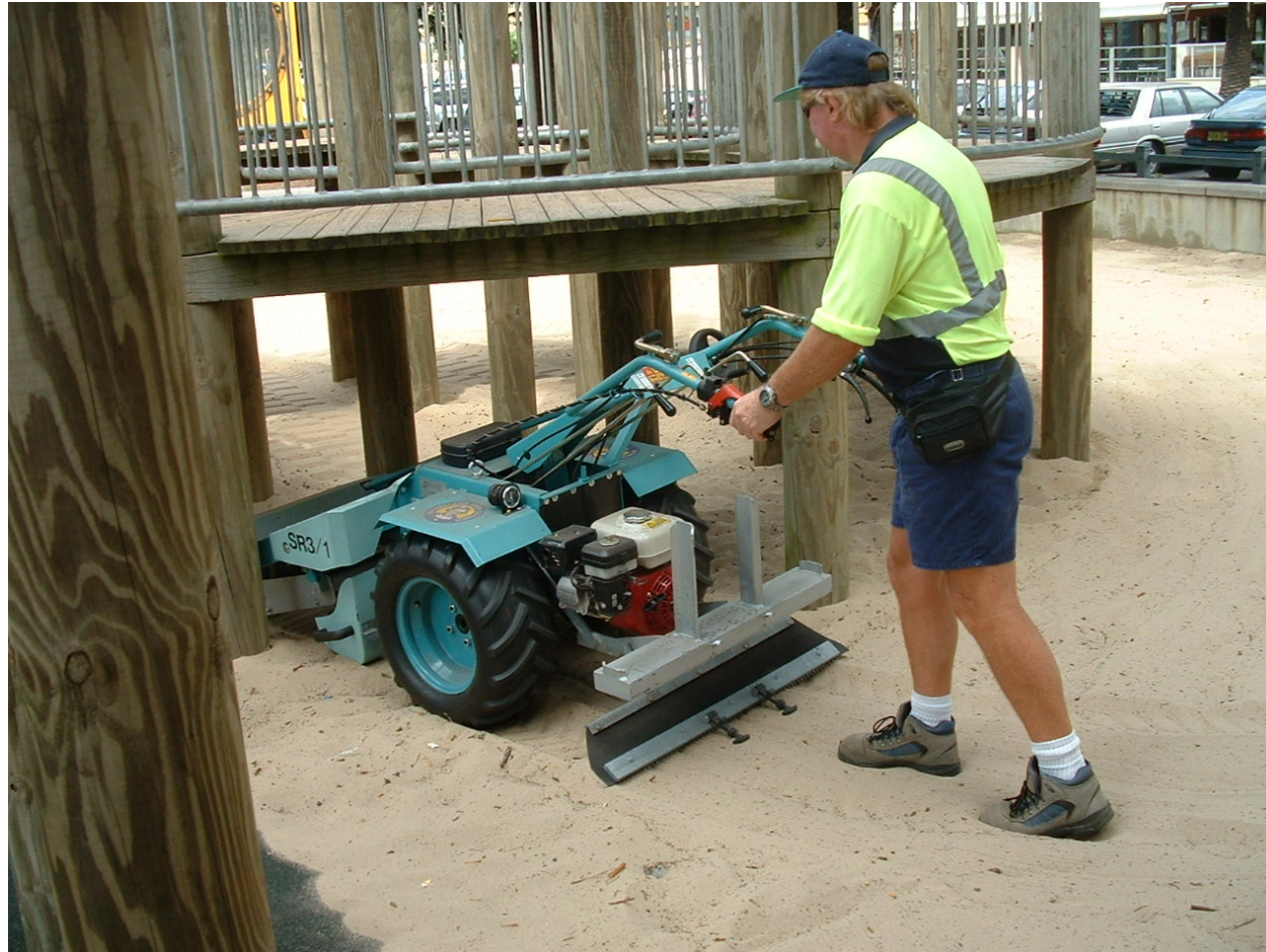
In-situ sieving using portable vibrating sieve
