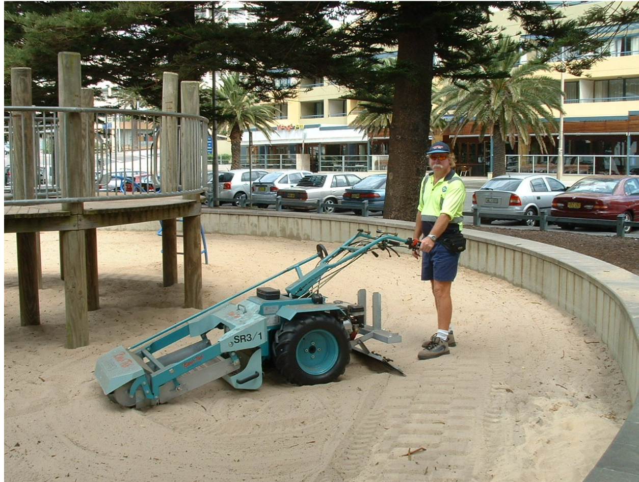
In-situ sieving using portable vibrating sieve
