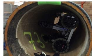
(b) Pipe assessment robot performing internal measurements.
