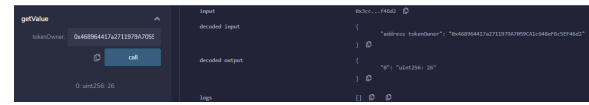
(a) The user with a valid token will only be permitted to check the value of the sensor
