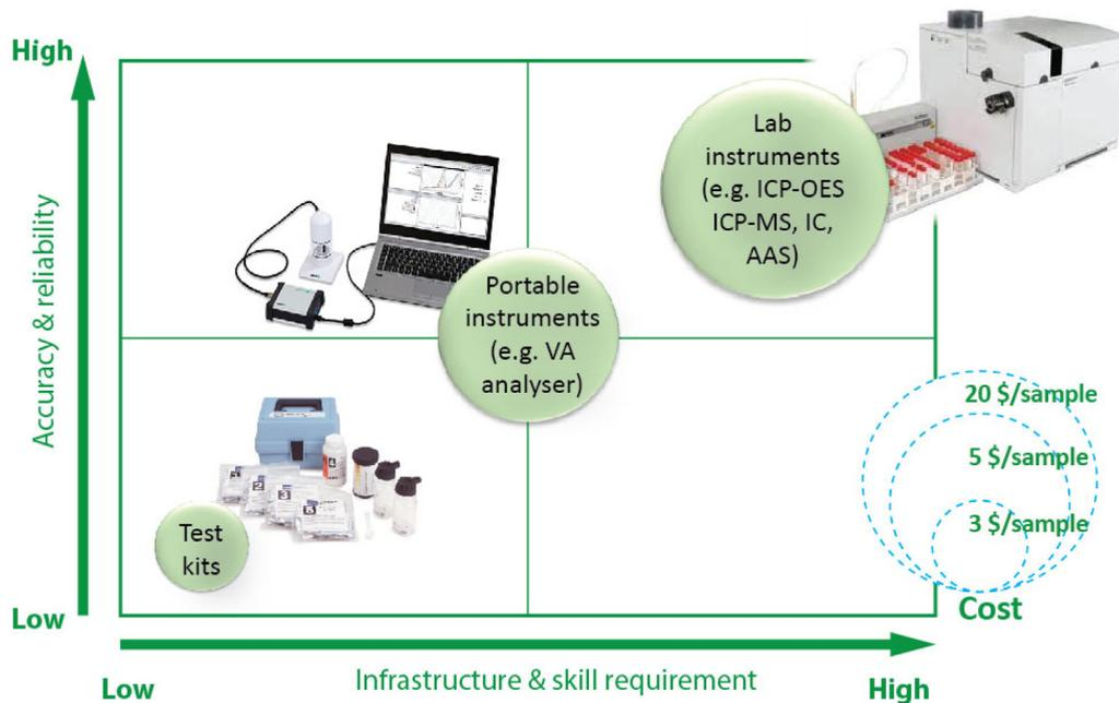
Fig. 3. Analytical techniques for quantifying arsenic in groundwater (the circle size is indicative of the cost of analysis).
