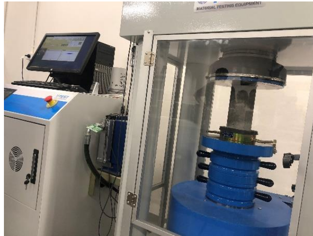
Figure 6: Concrete cylinder compression testing according to ASTM C39/C39M [26] in process at UTS Tech Lab
