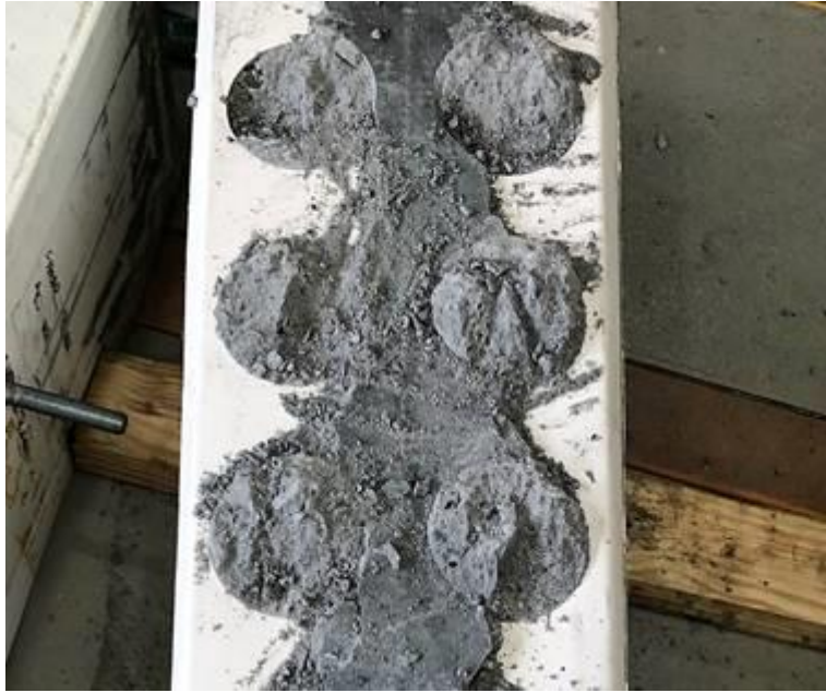
Figure 11: A Shear-BarChip failed interface
