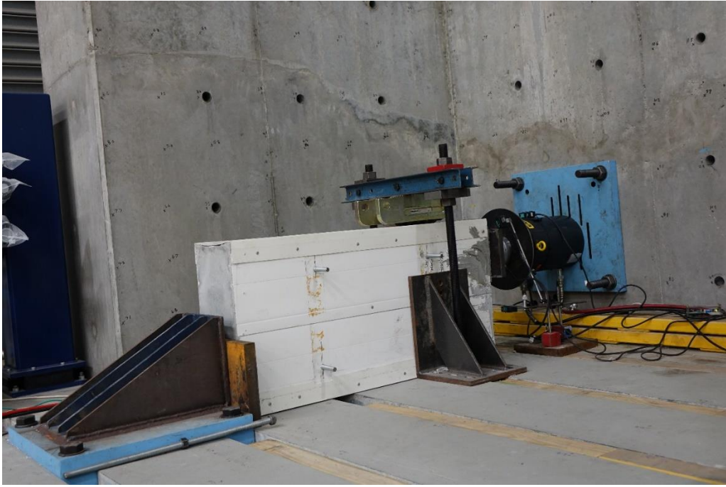
Figure 9: An overview of the direct shear test configuration at the Tech Lab
