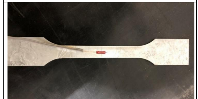
Fig. 3(b) Tensile coupon with strain gauge attached
