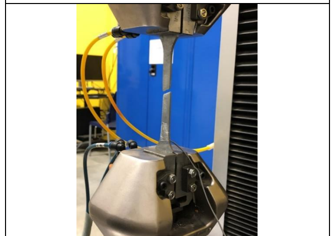
Fig. 3(c) Failure of CFS coupon during tensile testing
