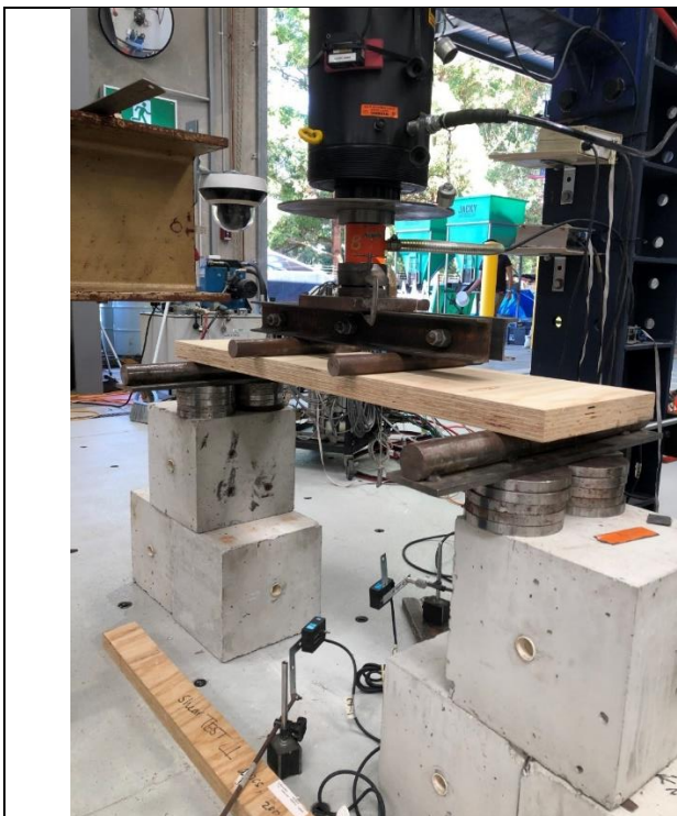
Fig. 6 Four-point bending test arrangement
