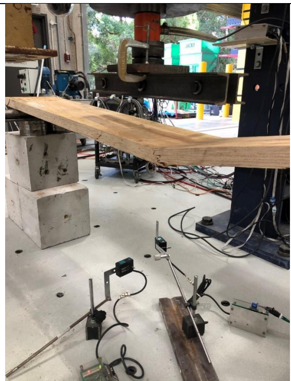
Fig. 7 Typical bending failure on tensile face of plywood panel
