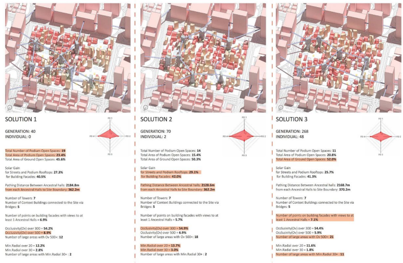
Figure 7. Results of third selection matrix. Solution 2 (middle) selected as the most optimal.
