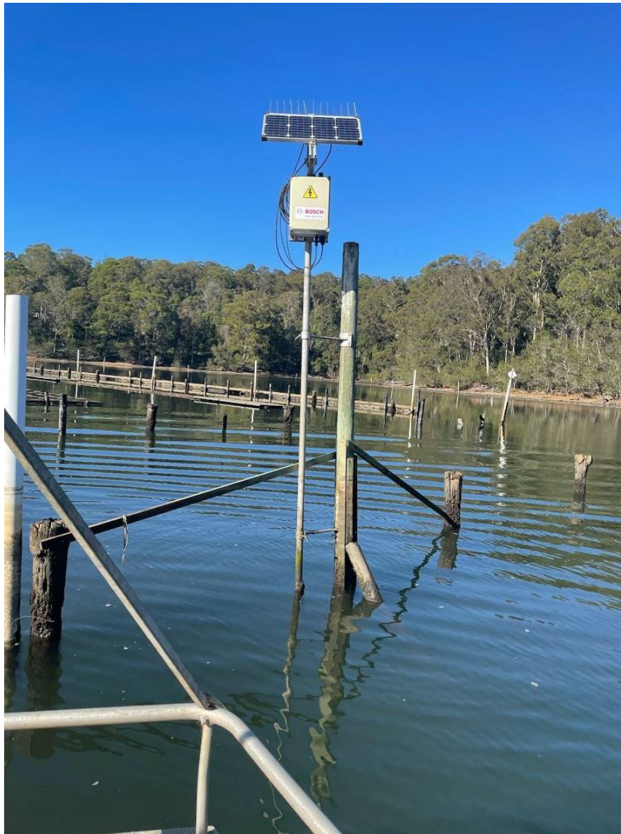
Figure A2 Seabird MicroCAT high accuracy conductivity, temperature and depth (CTD) field sensor deployed in Wagonga Inlet. Image: Brian Coxon.
