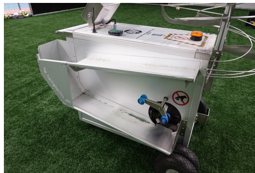
Figure 7. Ball Training Machine—ball-feeding mechanism.
