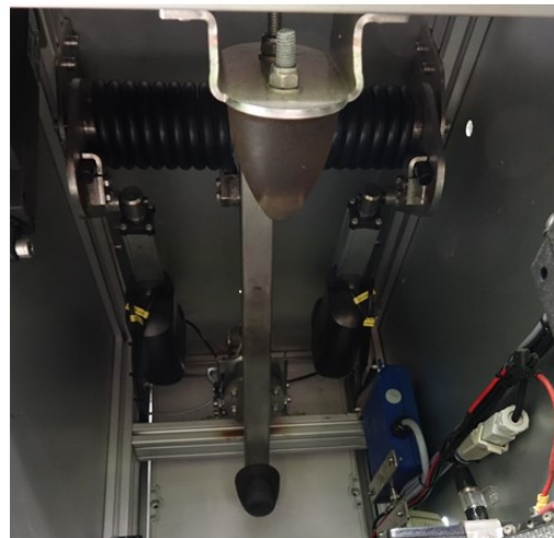
Figure 4. Ball Training Machine kicking mechanism.
