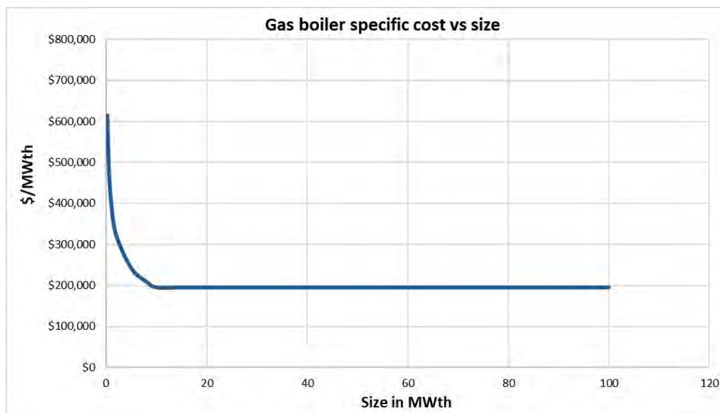
Figure 20: Gas boiler specific cost versus size.
