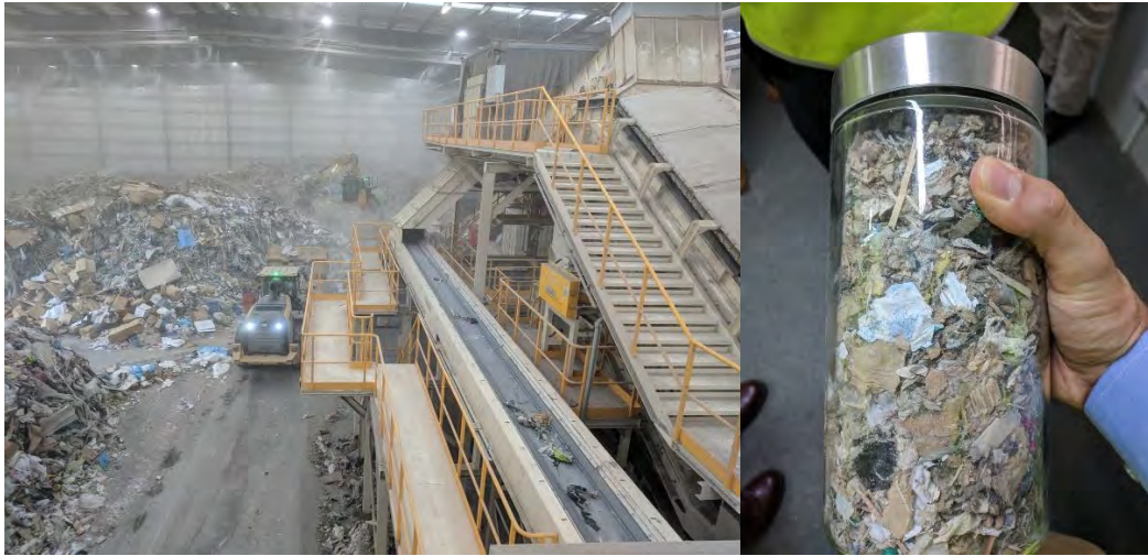
Figure 60. Waste treatment facility (left) and process engineered fuel product (right). (images ITP)
