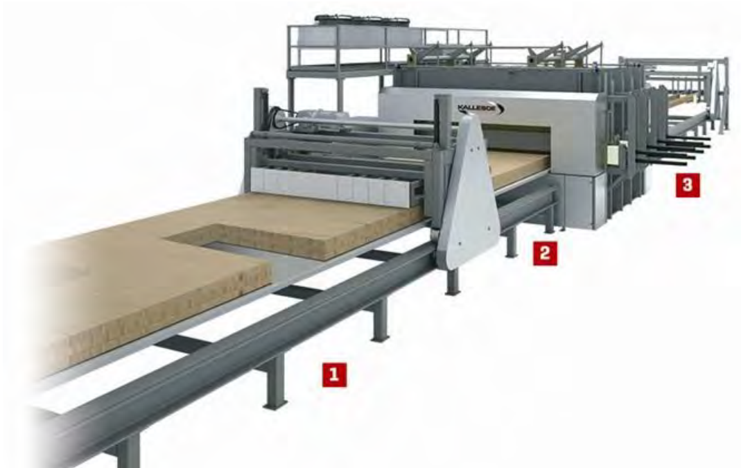
Figure 72: Kallasøe radio-frequency timber press (reproduced from: Kallasøe Machinery).
