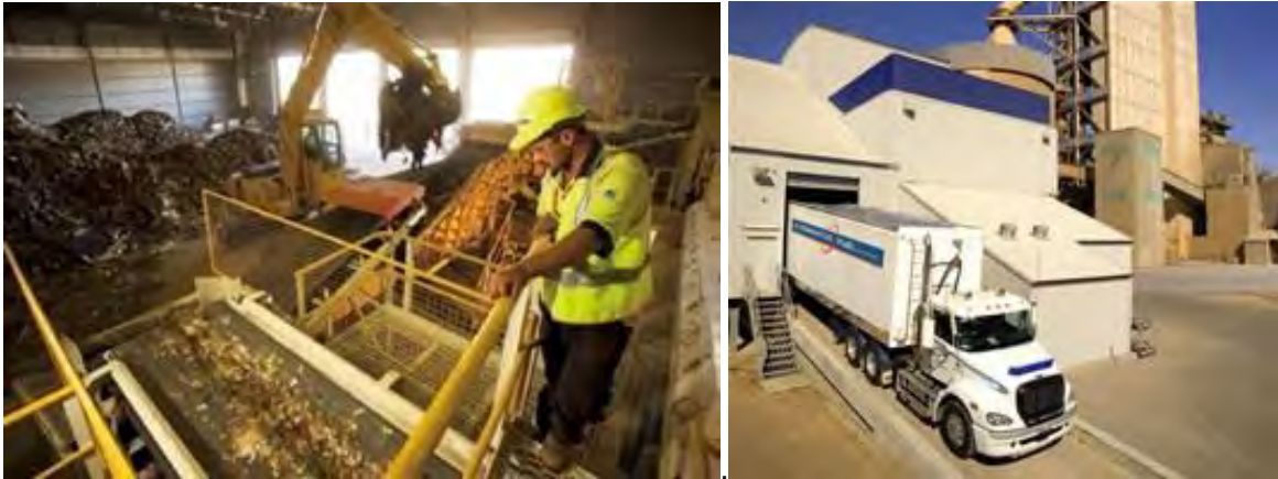
Figure 59: Construction and demolition timber processing and supply to the Birkenhead cement plant, (images Adelaide Brighton).
