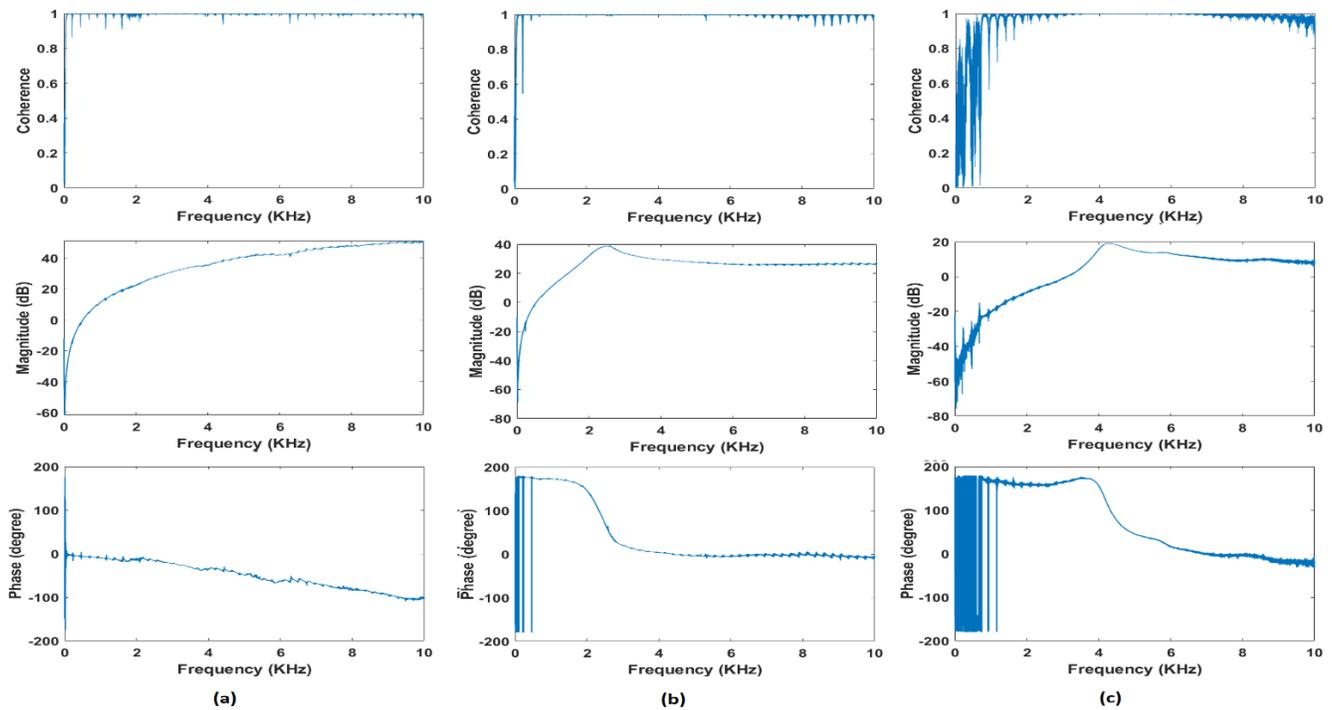
Figure 7: Coherence and frequency response function of the three actuators using the measured acceleration vs. voltage (a) P-841.10; (b) MTK12S18f25000; and (c) AB3342.
