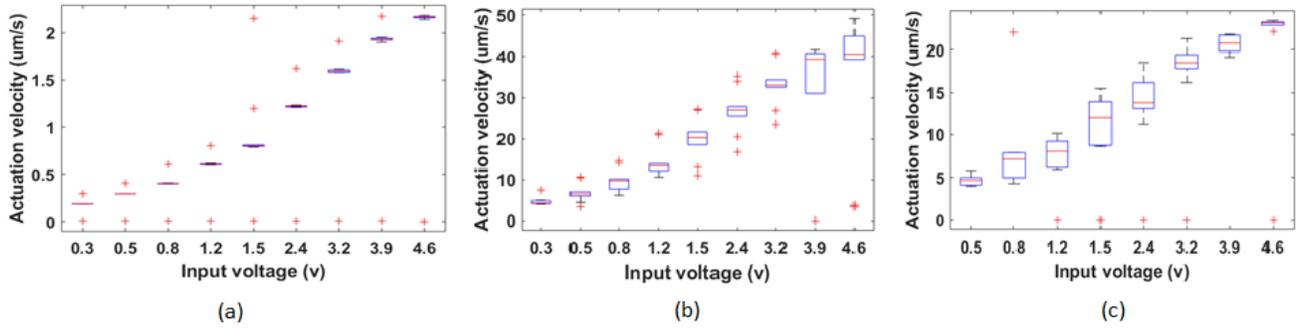
Figure 4: Linearity tests for the three actuators using the measured peak velocities for the voltage range of 0.3-4.6V for (a) P-841.10 (b); MTK12S18f25000; and (c) AB3342.
