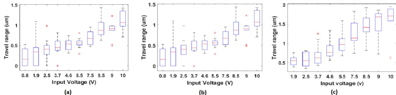
Figure 2: Displacement for three actuators (a) P-841.10; (b) MTK12S18f25000; and (c) AB3342.
