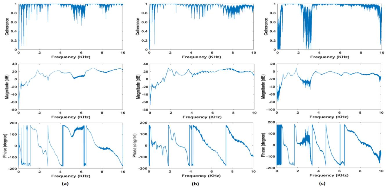
Figure 9: Coherence and frequency response function of Aluminium beam for the three actuators using the measured acceleration vs. voltage (a) P-841.10; (b) MTK12S18f25000; and (c) AB3342.
