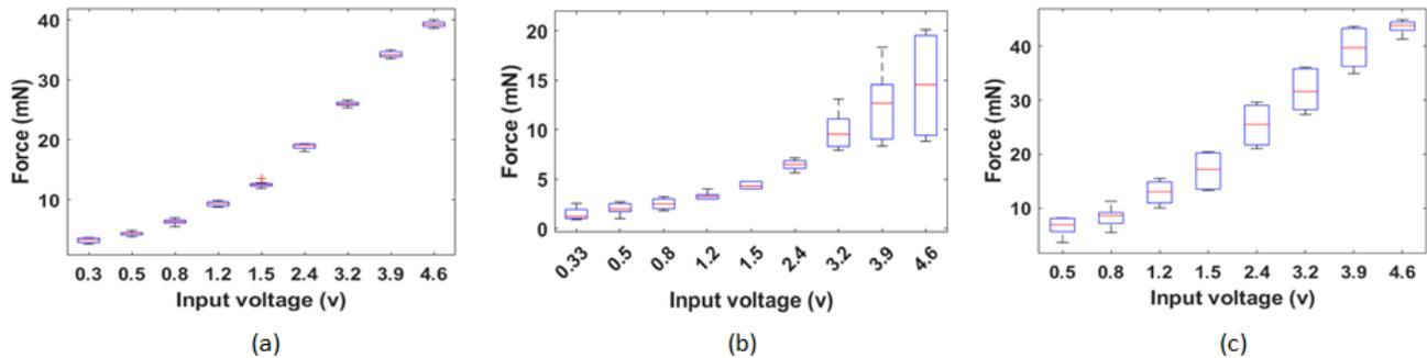
Figure 6: Linearity tests for the three actuators using the measured peak force for the voltage range of 0.3-4.6V for (a) P-841.10; (b) MTK12S18f25000; and (c) AB3342.
