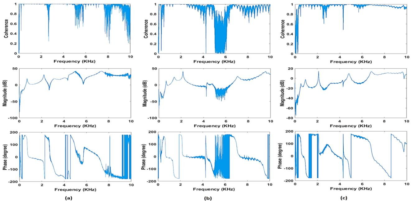
Figure 8: Coherence and frequency response function of Aluminium beam for the three actuators using the measured acceleration vs. voltage (a) P-841.10; (b) MTK12S18f25000; and (c) AB3342.
