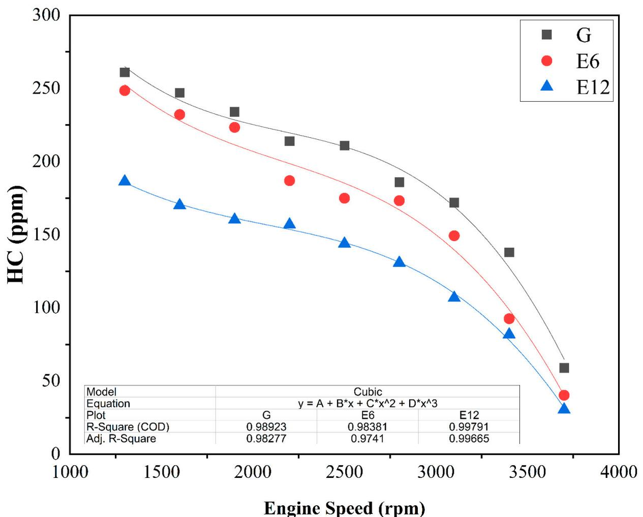
Figure 8. HC variation with engine speed.
