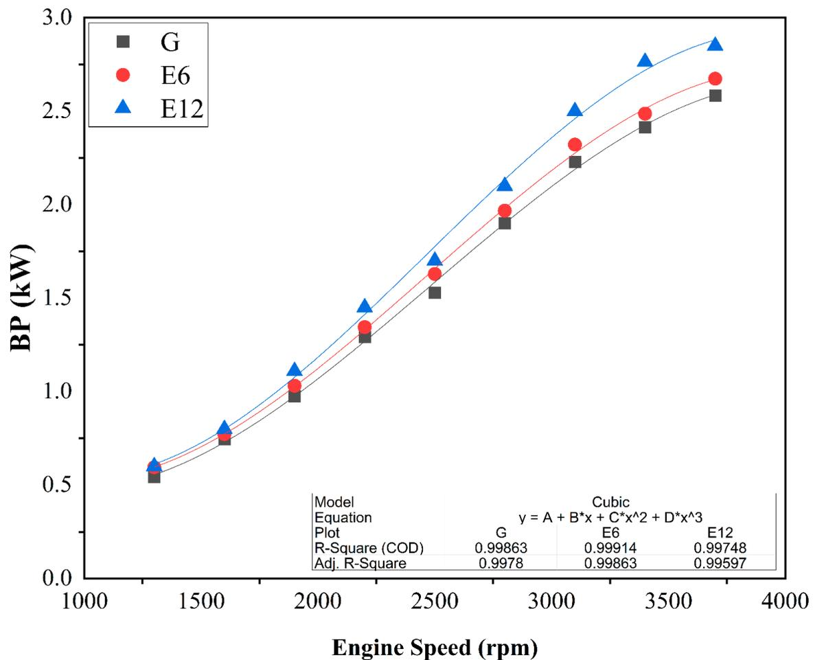
**Figure 3.** Brake power variation with engine speed.
