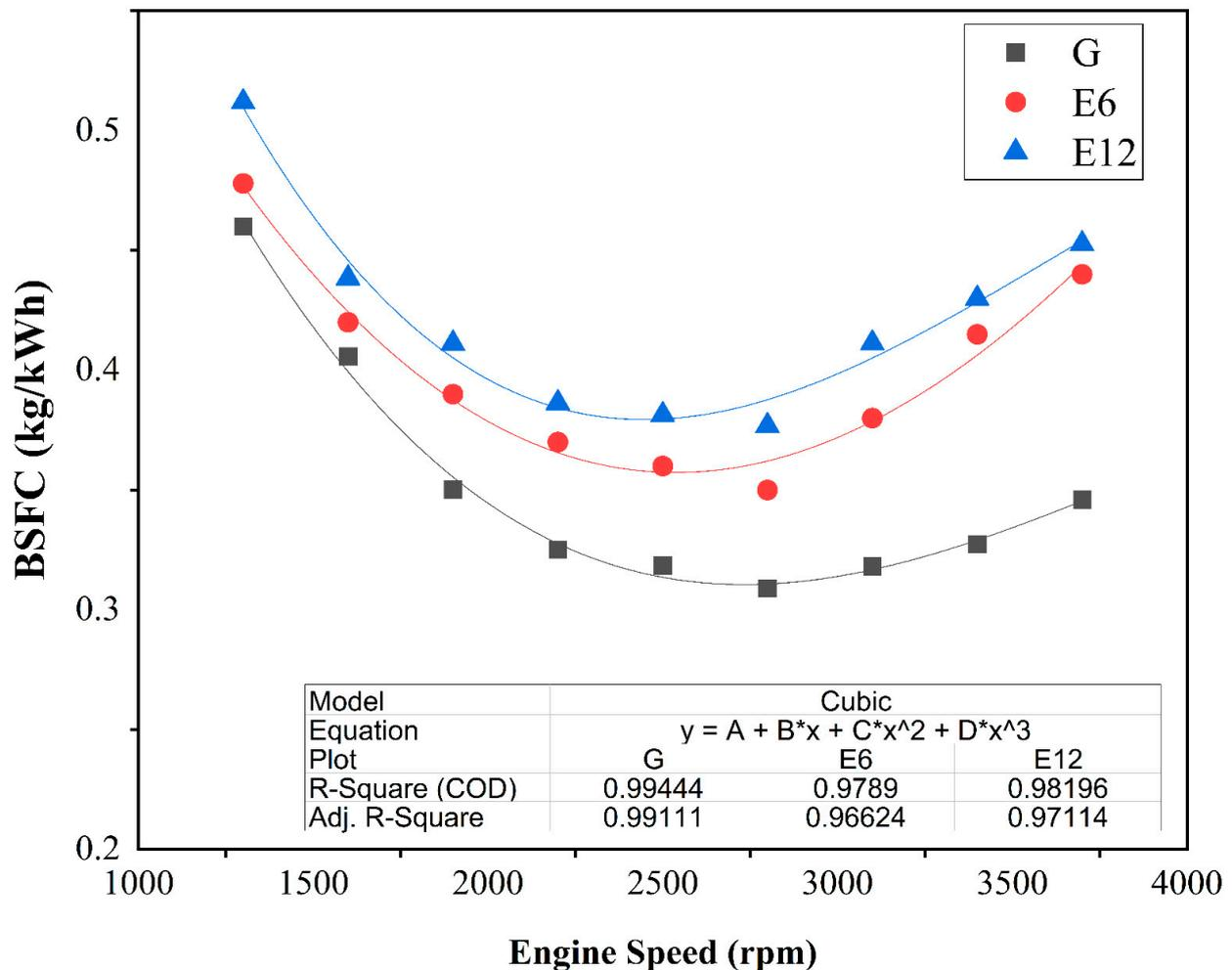
**Figure 4.** BSFC variation with engine speed.
