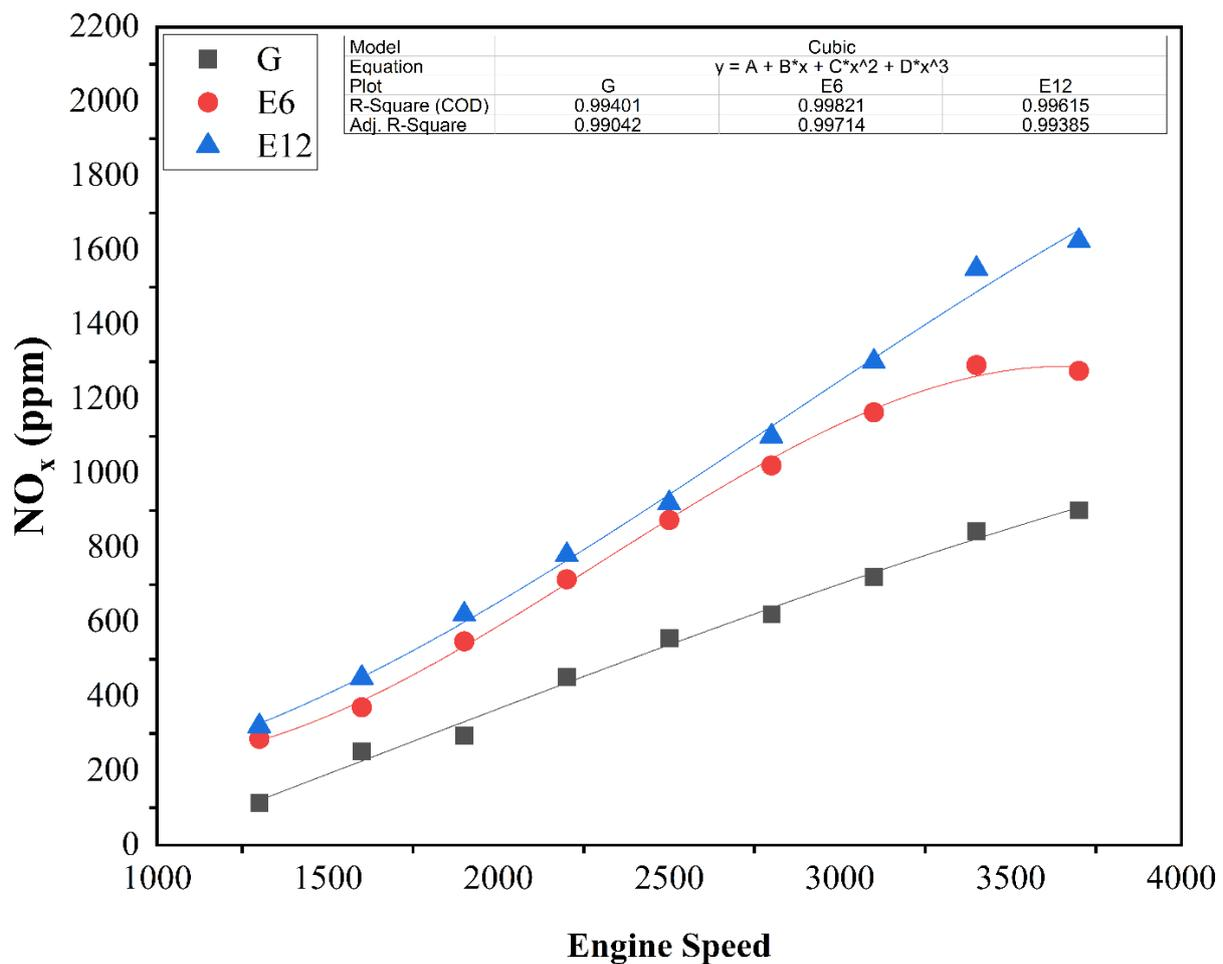
**Figure 9.** NO<sub>x</sub> variations with engine speed.
