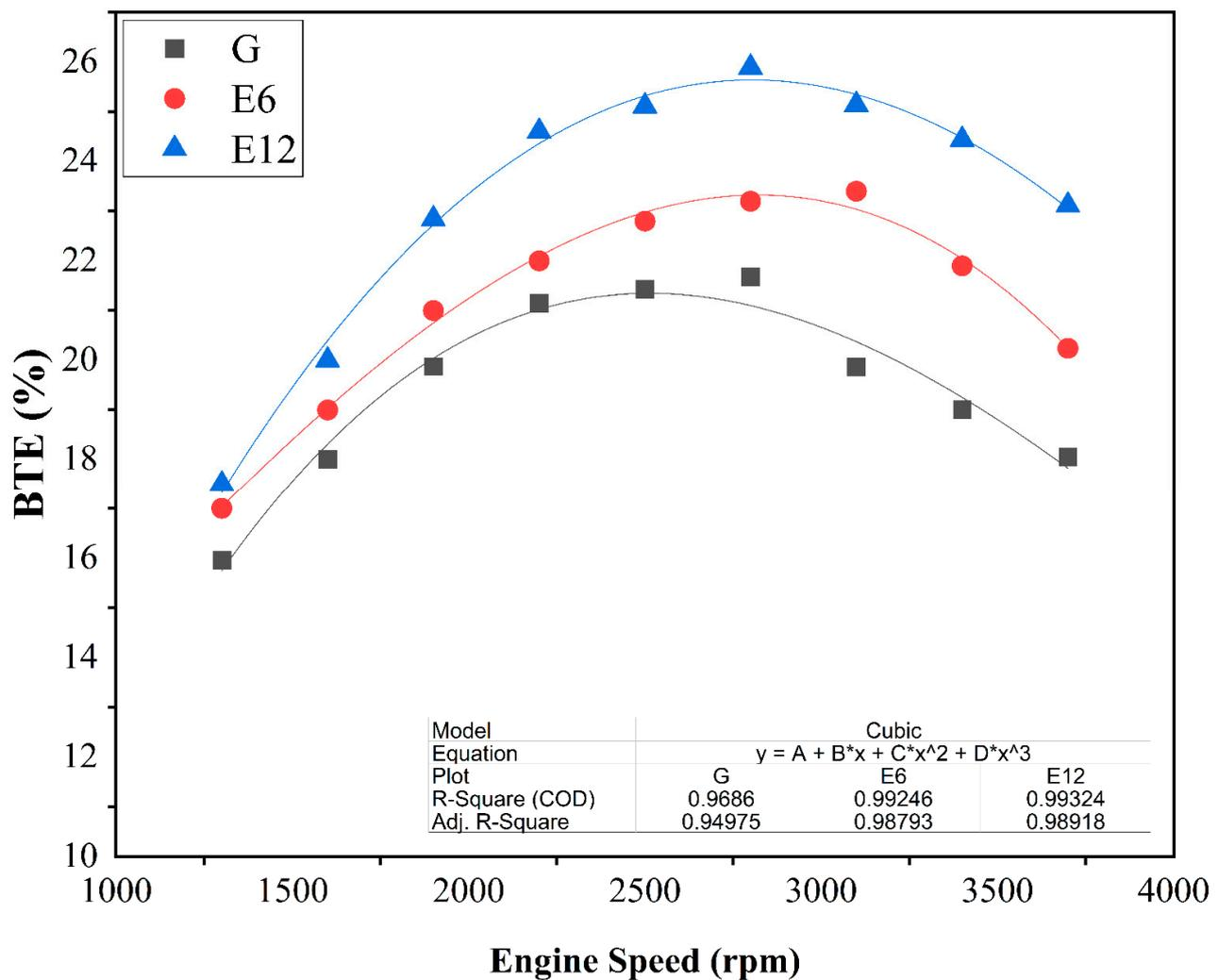
Figure 5. BTE variation with engine speed.
