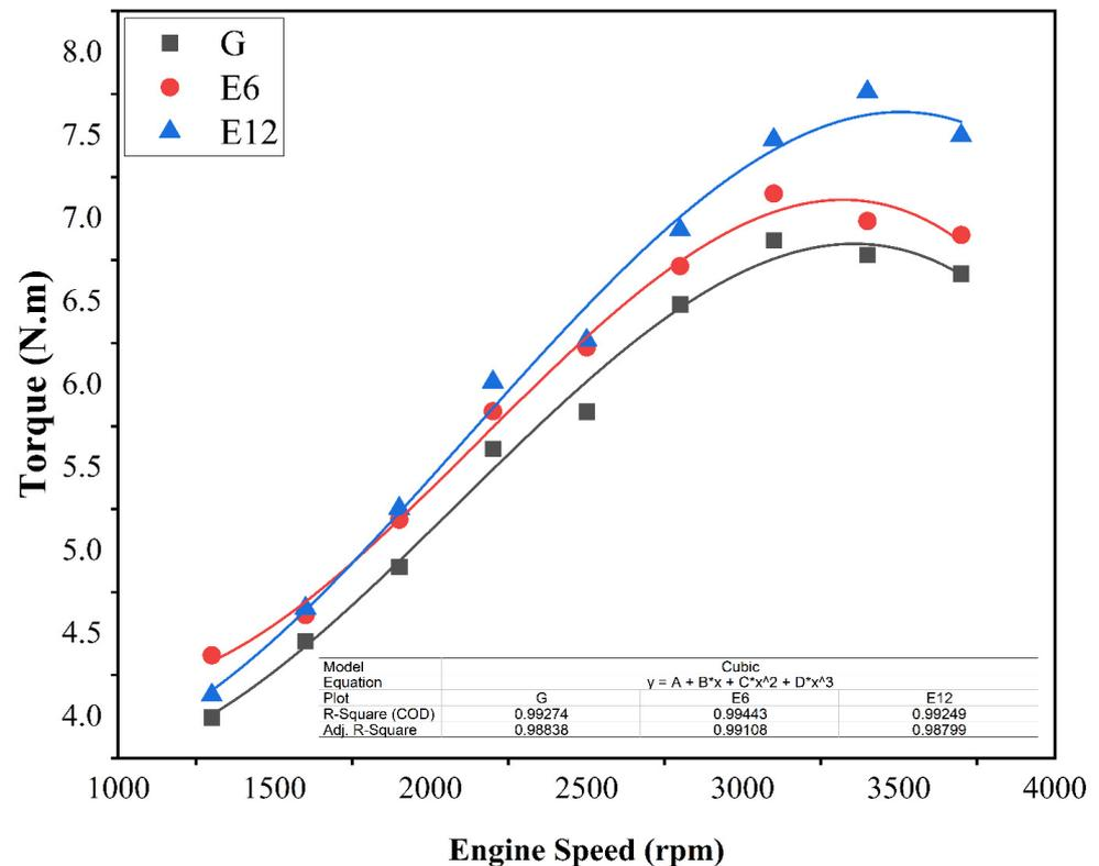
Figure 2. Torque variation with engine speed.
