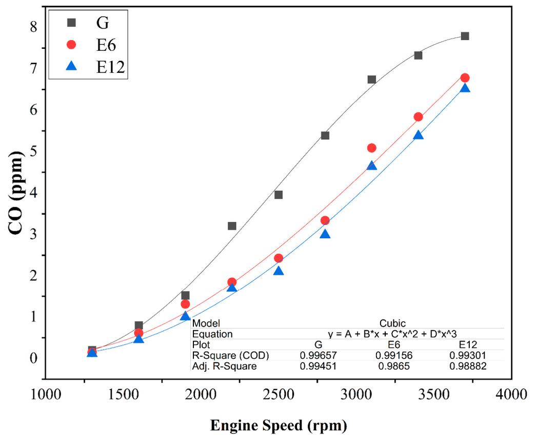
Figure 6. CO variations with engine speed.
