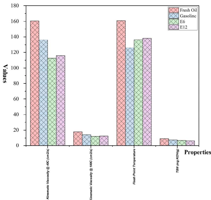
**Figure 10.** Comparison of lube oil properties.
