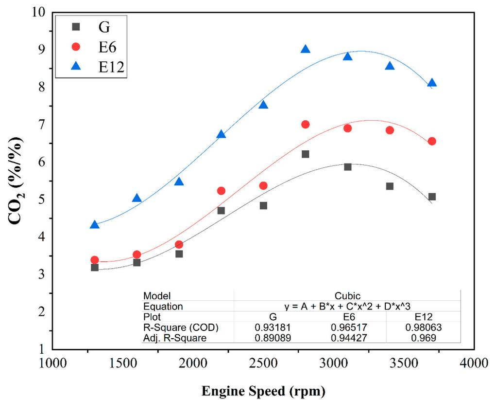
Figure 7. CO<sub>2</sub> variation with engine speed.
