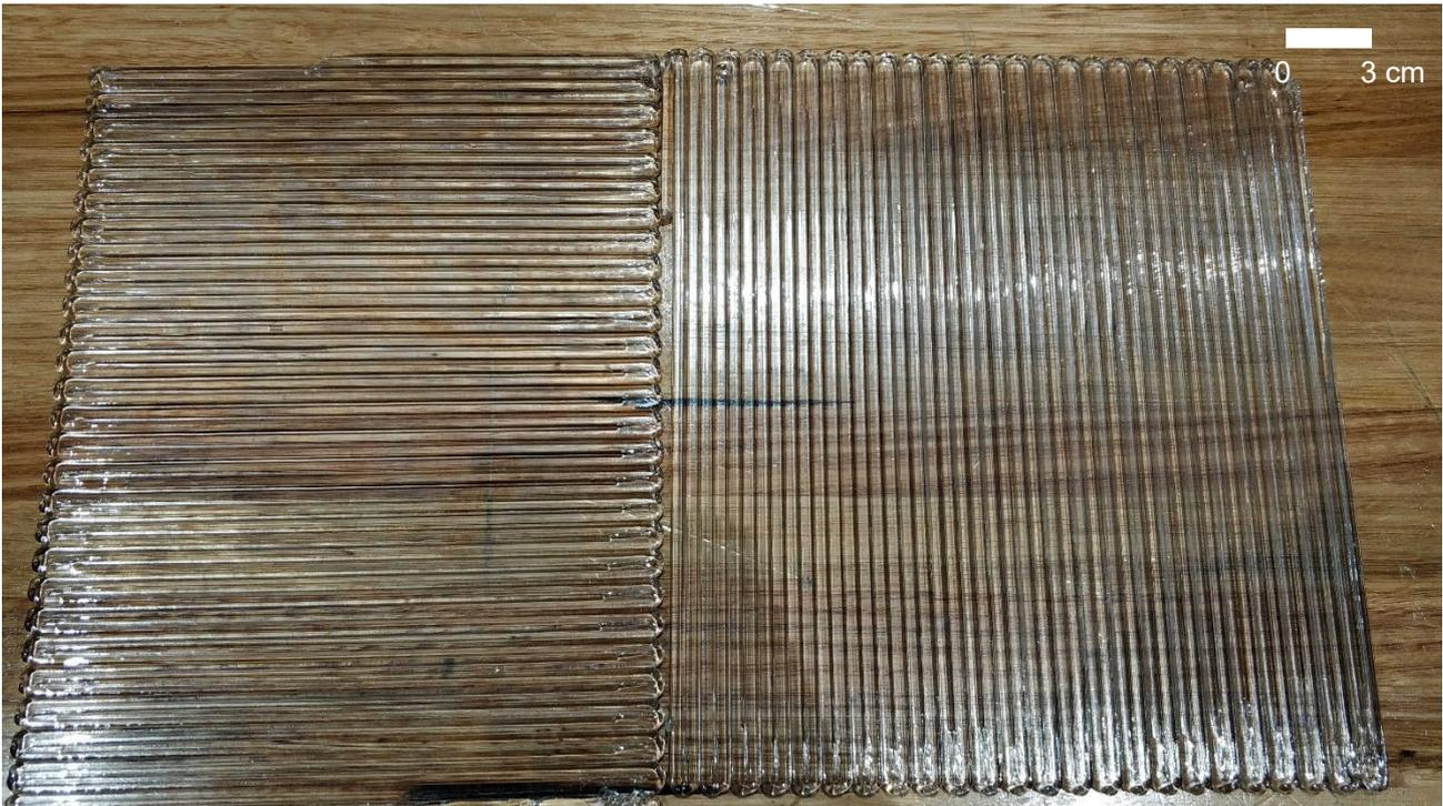
**Figure 6: The printed base shapes for the  $E_1$  and  $G_{12}$  tensile samples**
