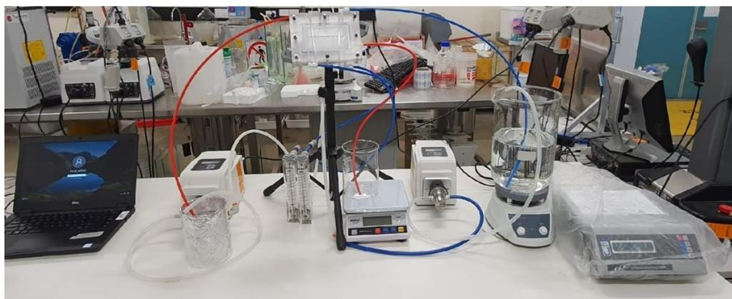
**Figure A1.** Schematic diagram of the AGMD setup.
