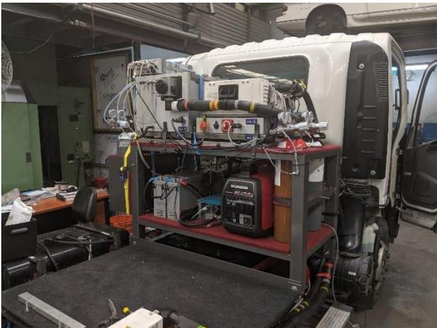
Figure 2. PEMS installation on the hydraulic hybrid truck.
