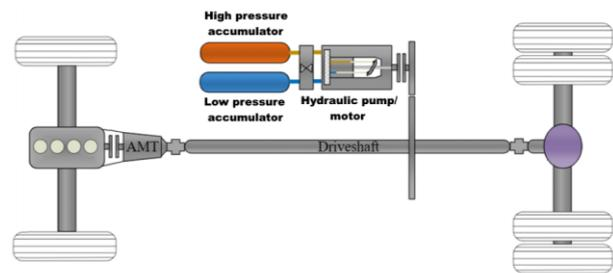
Figure 1. Powertrain architecture for the hydraulic hybrid driveline. Figure adapted from Zhou (2021) with permission.
