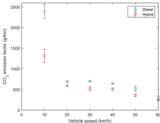
Figure 6. Speed-dependent emission factors for CO<sub>2</sub> in diesel and hybrid mode derived from the urban test route. Data are binned according to speed based on 1 Hz emission data. Data are pooled across cold start and hot running conditions.
