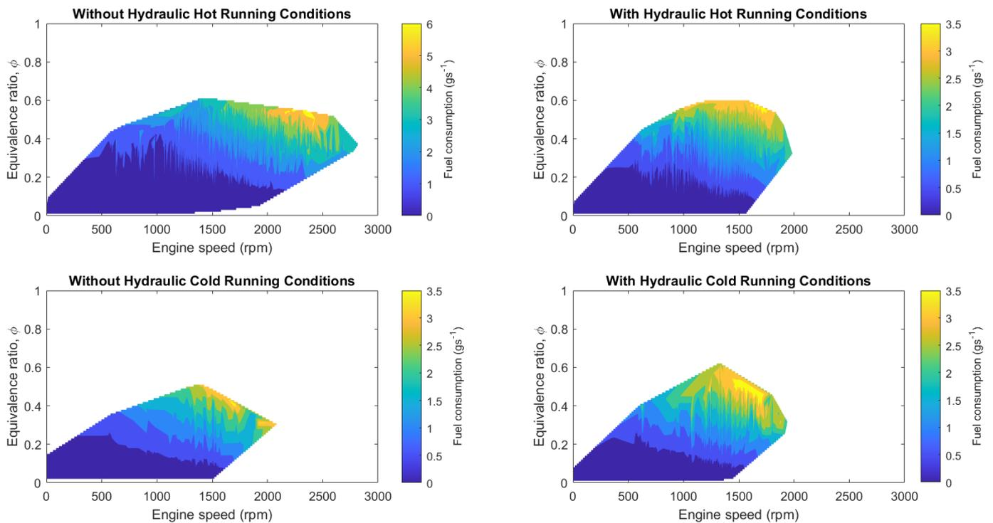
Figure 5. Engine maps for fuel consumption during both hot and cold running conditions for conventional diesel operation and for hybrid mode.
