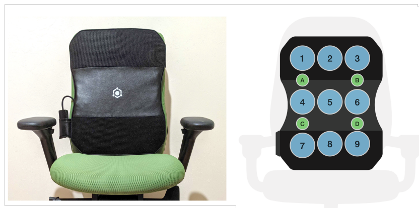
Figure 2. Front view of the LifeChair interface (left) and the LifeChair sensor layout (1 to 9) (right).
