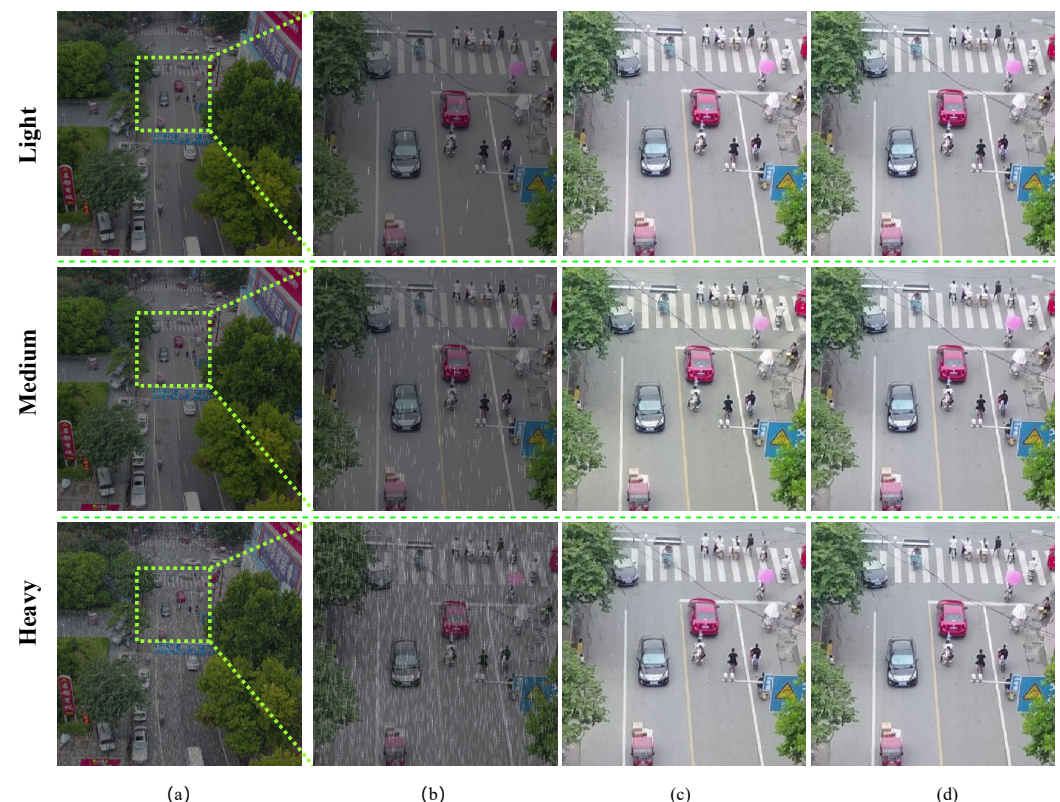
Figure 11. Visualization of images and patches reconstructed by Deraining Subnetwork. (a) The original input images. (b) The patches cropped from the original image. (b) The reconstructed rain-free patches. (c) The corresponding ground truth.
