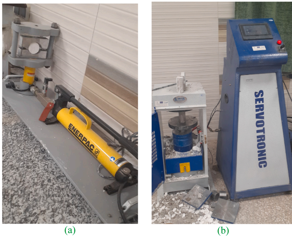
Fig. 4. a) Brazilian test machine, b) uniaxial test machine.
