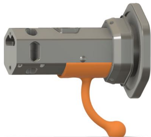
Figure 19. 3D printed mounting device to ensure microphone position when mounted horizontally (shown with windscreen on).
