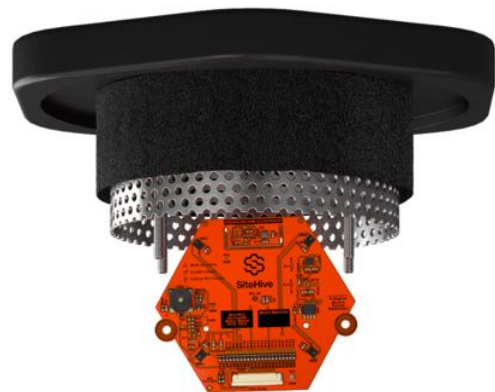
Figure 11. Design candidate windscreen 1, noiseboard for scale reference (deployed as horizontal plane).
