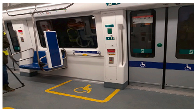
Fig. 10. Improved reserved areas for PwD. Implementation of sensor technology to avoid accidents when entering the trains.
