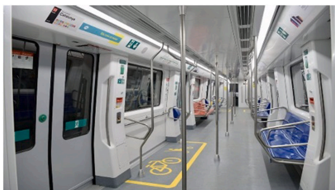
Fig. 8. Improved signage and areas for PwD where the areas for bicycles and prams have been clearly separated from the reserved seating for PwD.
