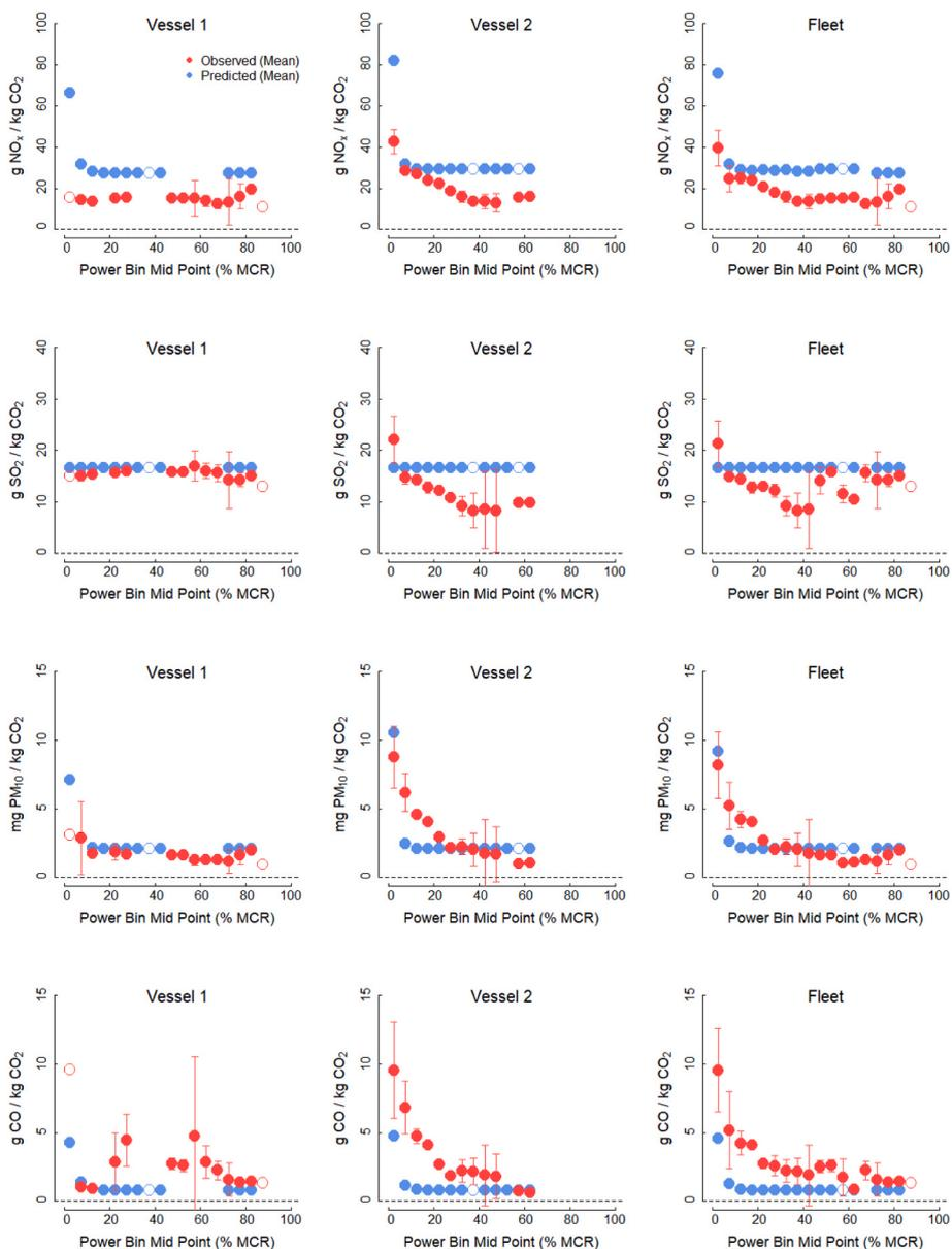
**Fig. 5.** Measured and predicted emission ratios for four air pollutants, two levels of aggregation and twenty power bins, including the 95% confidence intervals for measured emission factors and the range (min-max) for predicted emission factors. Open dots represent bins with only one value.
