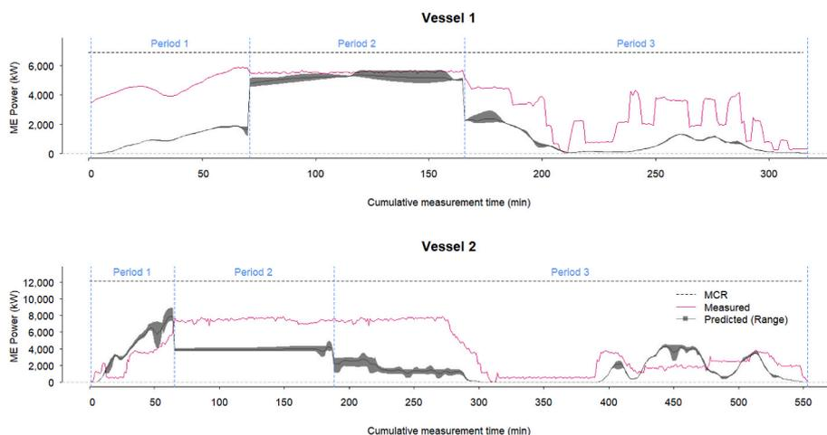
**Fig. 4.** Measured on-board power and the range of estimated main engine power using different AIS post-processing methods in cumulative minute time steps, vertical dotted blue lines demark the three different measurement periods for each ship. (For interpretation of the references to colour in this figure legend, the reader is referred to the Web version of this article.)
