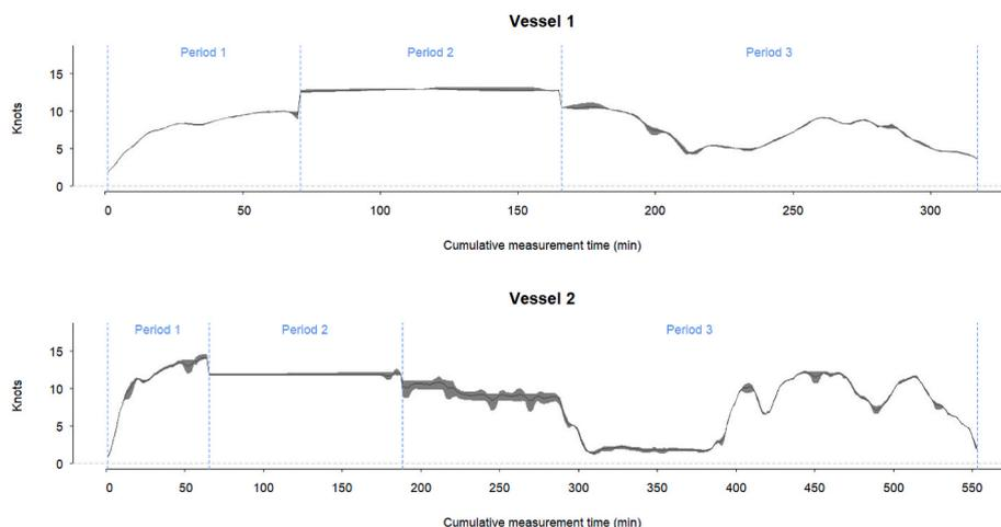
**Fig. 3.** The range of estimated vessel speeds using different AIS post-processing methods in cumulative minute time steps, vertical dotted blue lines demark the three different measurement periods for each ship. (For interpretation of the references to colour in this figure legend, the reader is referred to the Web version of this article.)
