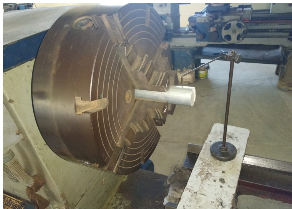
Figure 7. Centering of workpiece.
