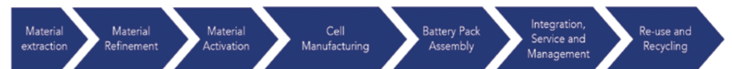
Figure 11 Battery Production Process
