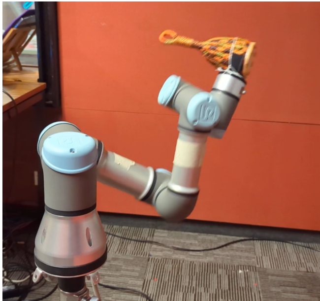
Figure 1: UR3 Robot arm imitating a human percussionist playing a caxixi (percussion instrument).
