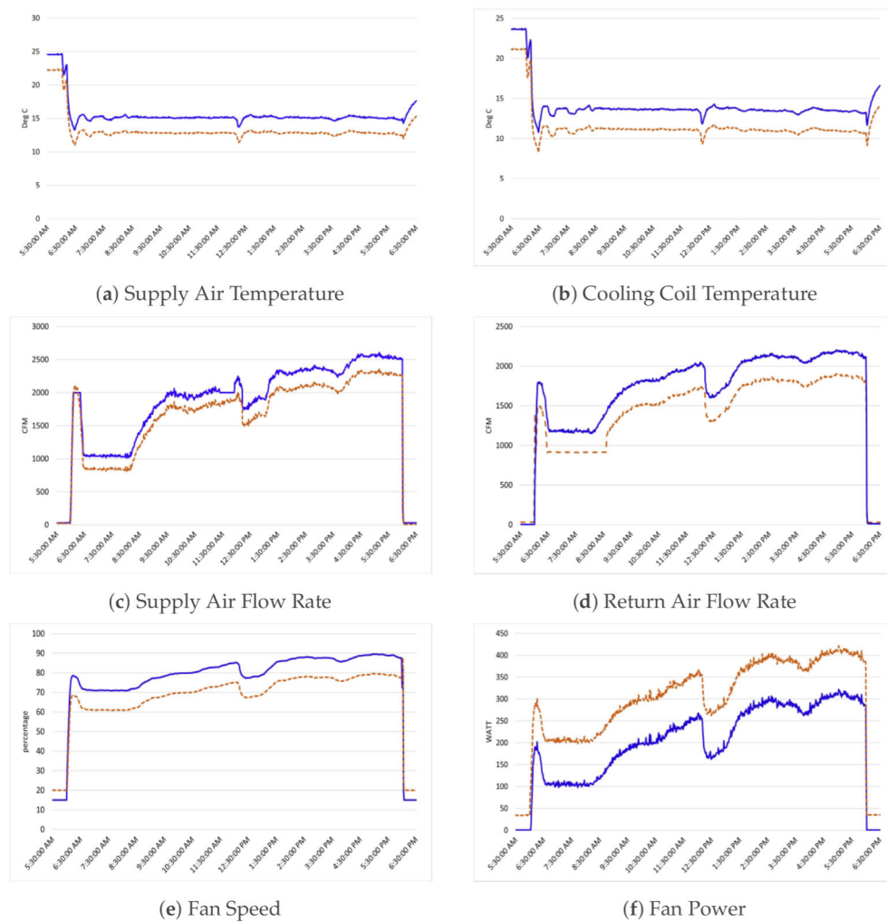
Figure 2. Comparison analysis of simulated and ASHRAE HVAC operation data [26]. (— HVAC-SIM+ Simulated Data; - - - ASHRAE Data).
