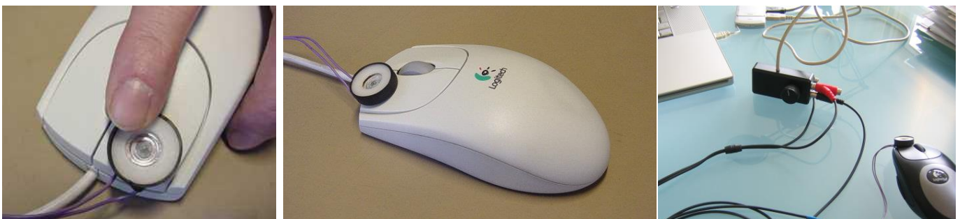
Figure 2. The vibrotactile element in position, on the mouse used in the experiments reported in this paper ( left and middle ), and a later version on a newer mouse and computer ( right ).
