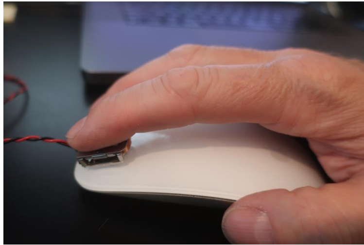
Figure 6. The current set-up using a small surface transducer for improved tactual feedback.
