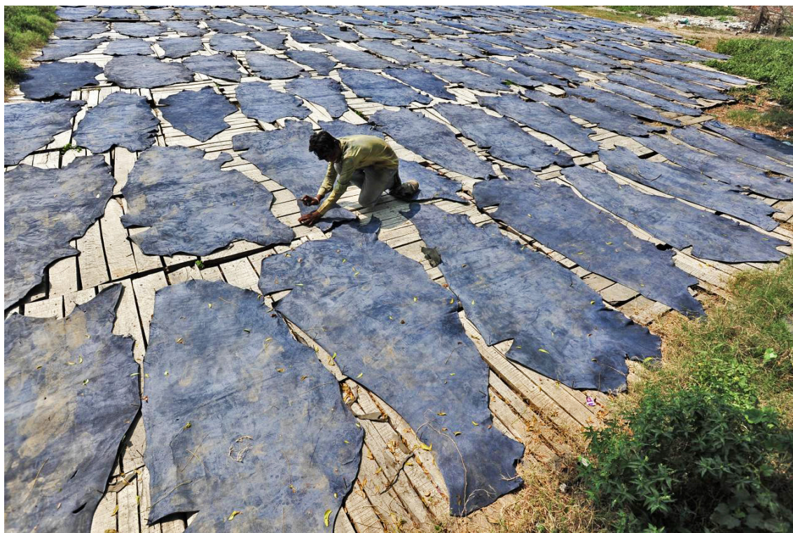
Leather hides drying in the sun in Kanpur, India. Chrome tanning is the most prevalent method practiced worldwide, but chromium is highly toxic. Untreated wastewater from the tanning process can release a witches' brew of chemicals into the environment including heavy metals such as cadmium, lead and arsenic. Image by Neil Palmer/IWMI Flickr Photos via Flickr (CC BY-NC-ND 2.0).
