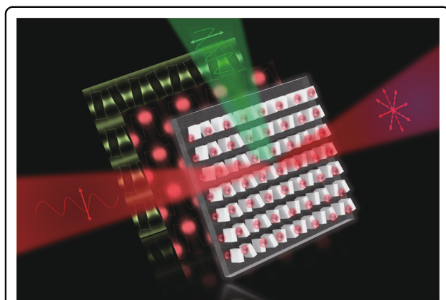
Fig. 1 Upconversion emission enhancement with polarization control. A 980 nm laser beam is directed into a non-rotationally symmetric arrangement of nanobricks comprising an all-dielectric metasurface. Through the interplay of QBIC resonance (green pattern) and Mie resonance effects (red pattern), upconversion nanoparticles (pink spots) coated onto the surface of the nanobricks exhibit enhanced fluorescence emission with directional polarization controls
