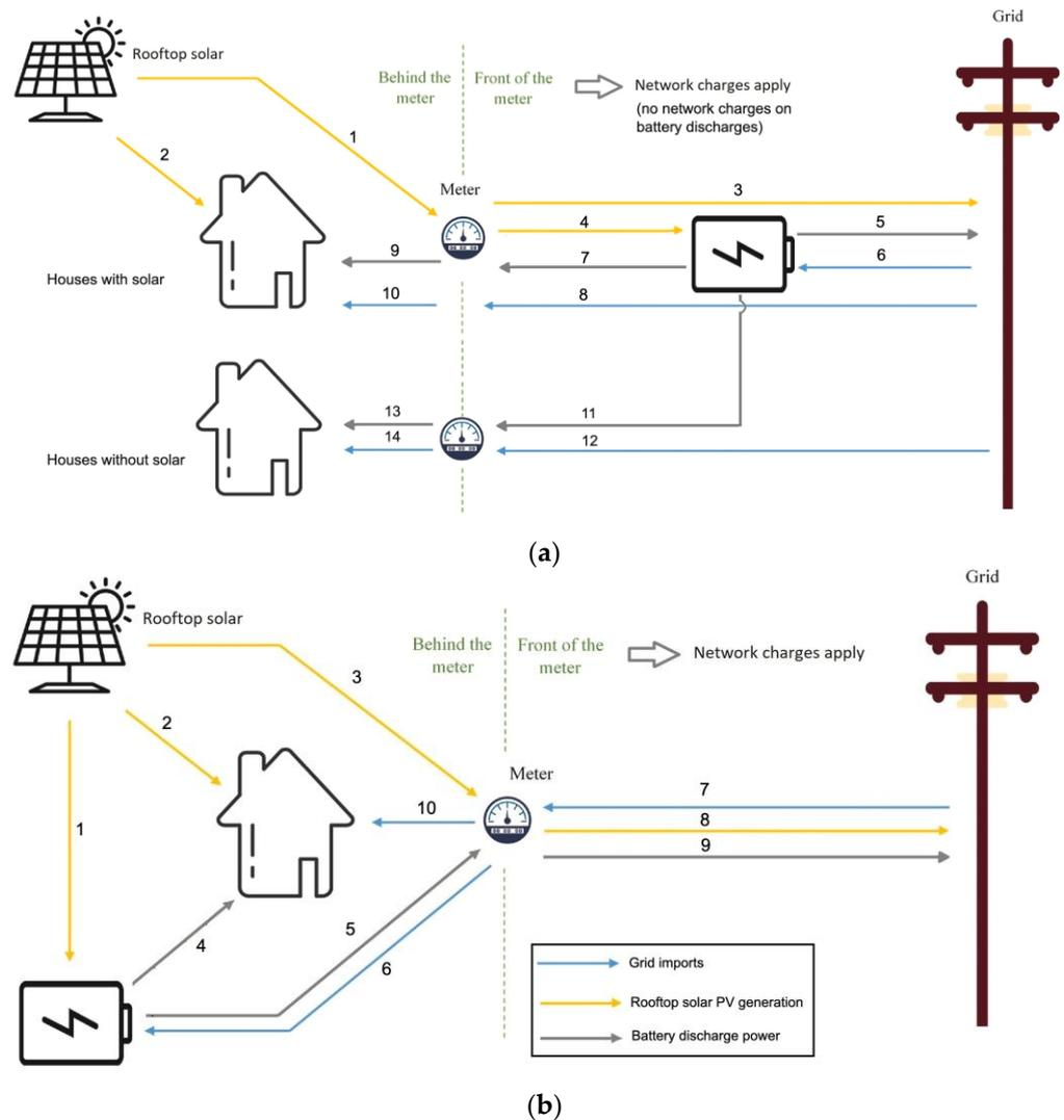
**Figure 2.** Comparison of the energy flows in (a) FTM and (b) BTM batteries (adapted from [76]).
