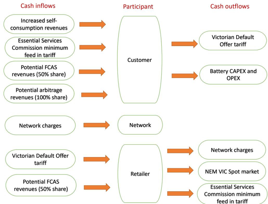
**Figure 4.** Participant-level value flow configurations in the BTM battery model.
