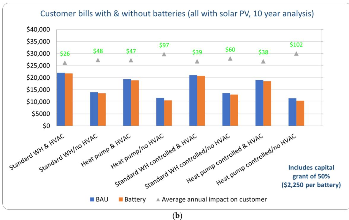
**Figure 8.** Impact of BTM batteries (1-h energy storage) on electricity bills for various PV-equipped households: (a) without grant and (b) with 50% grant.
