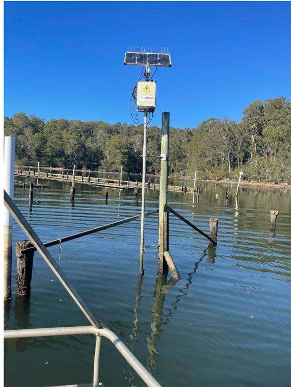
**Figure A2** Example of a Seabird MicroCAT high accuracy conductivity, temperature and depth (CTD) field sensor deployed in NSW estuaries.
