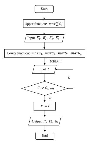
Figure A1. Bi-level multi-objective optimization model algorithm flow.
