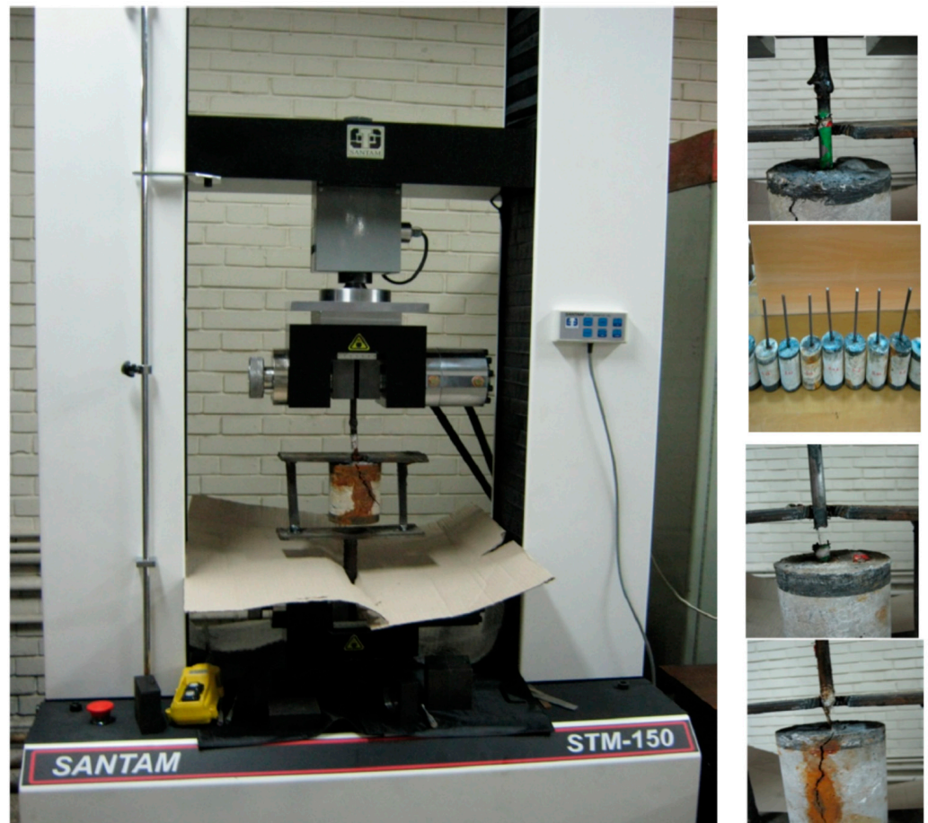
Figure 2. Pullout of steel–concrete bond joints test apparatus.
